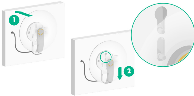
Figure 2-7 Attaching the AP to the mounting bracket
