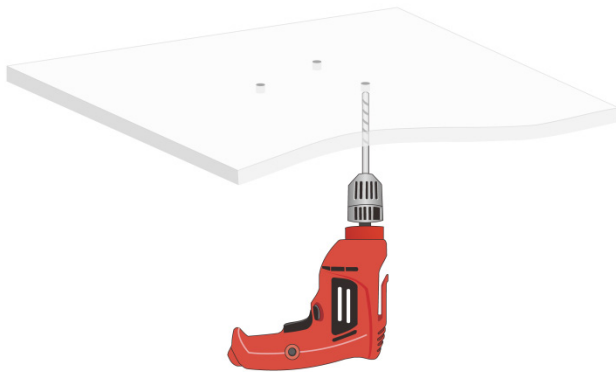
Figure 2-8 Drilling holes in the ceiling tile
