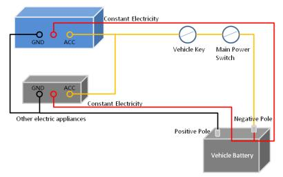
Figure 2-9 Vehicle main switch installed on the negative pole of the vehicle battery
