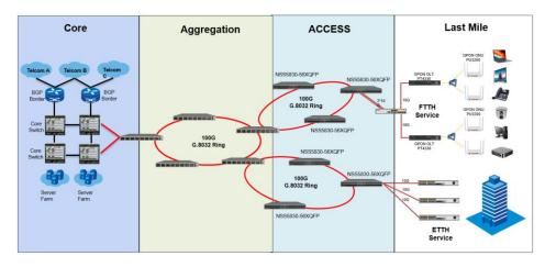
With the rapid growth of triple-play services, higher requirements are put forward for the performance, bandwidth and quality of the ISP Metro Ethernet networks. The NSS5830 series 100G switch have been developed to meet the increasing demand of FTTx services for ISPs. The NSS5830 series provide up to 8-Port 100G interfaces for building backbone network. It will greatly increase the bandwidth and improve the internet experience of end users.
