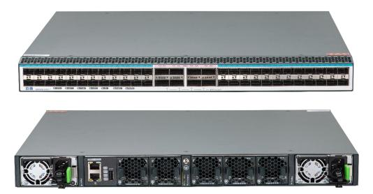
NSS5830-56XQFP supports 48\*10G SFP+ optical interfaces, 8\*100G QSFP28 optical interfaces, five modular fan slots and dual modular power slots.
