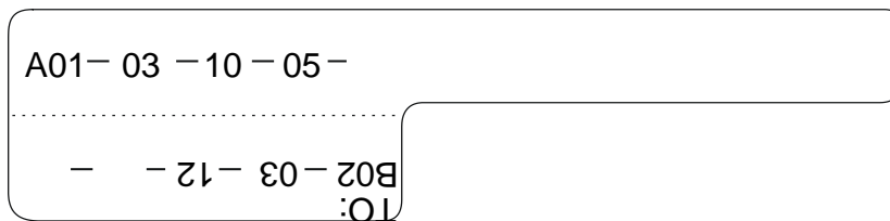
Figure10-9 Example of a label on an Ethernet cable
