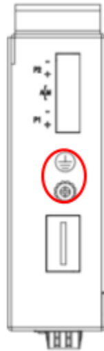
Figure 4 — The grounding screw on the switch
