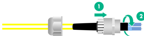
Figure2-11 Fastening the weatherproof connector
