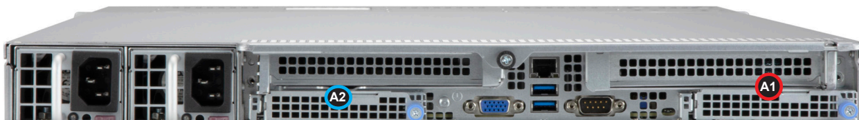
Figure 3-12. AIOM Chassis Slots
