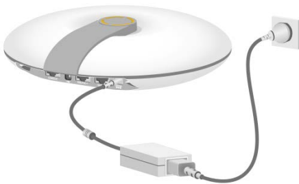
Figure2-14 Using a power adapter to connect the AP to a local power source
