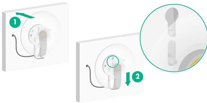
Figure2-7 Attaching the AP to the mounting bracket
