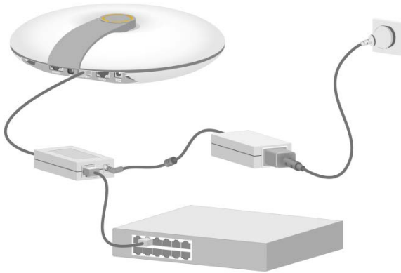
Figure2-15 Connecting a power injector
