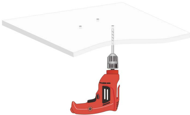
Figure2-8 Drilling holes in the ceiling tile
