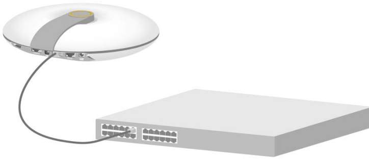
Figure2-13 Powering the AP through PoE
