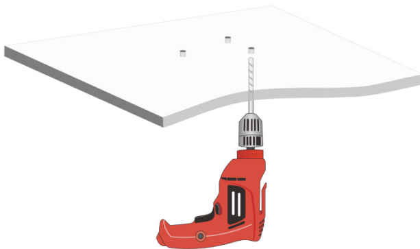
Figure2-10 Drilling holes in the ceiling tile
