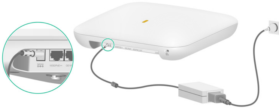
Figure2-15 Using a power adapter to connect the AP to a local power source
