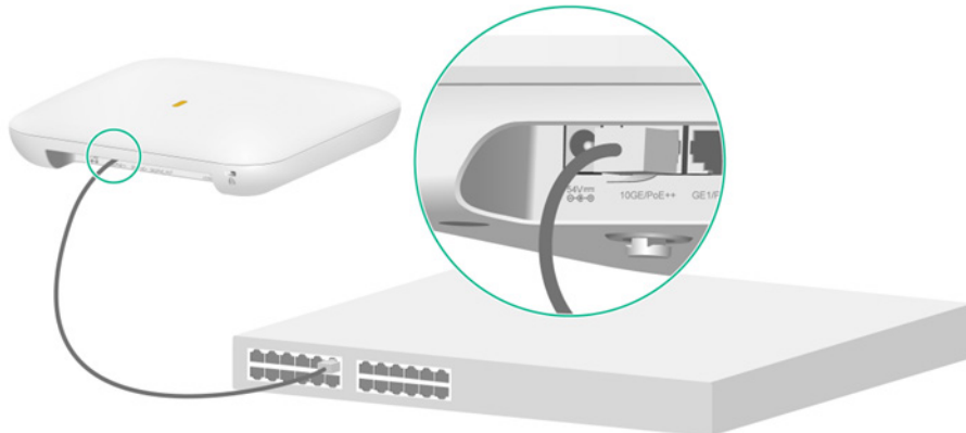
Figure2-14 Powering the AP through PoE
