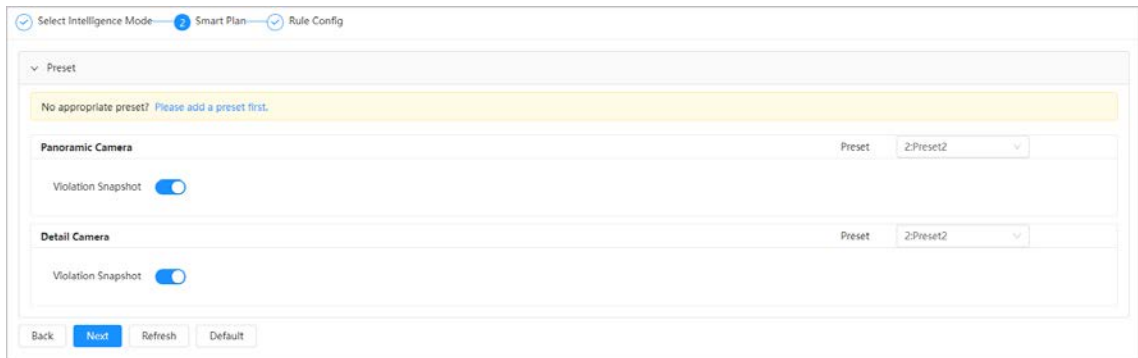
Figure 8-4 Enable violation snapshot (combination mode)
