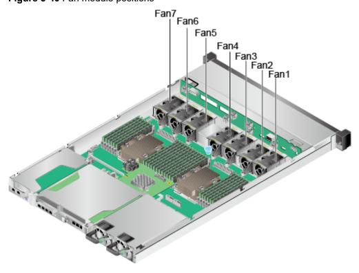
Figure 5-40 Fan module positions
