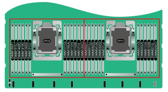
Number of DIMMs (√: recommended o: not recommended) CPU Channel **DIMM Slot** ✓ 0 ✓ 0 0 1 2 3 4 5 6 7 8 9 10 11 12 DIMM000(A) A DIMM001(G) • • DIMM010(B) В • • DIMM011(H) DIMM020(C) C DIMM021(I) • CPU 1 DIMM030(D) D DIMM031(J) • • • • DIMM040(E) E DIMM041(K) • • DIMM050(F) F DIMM051(L)
