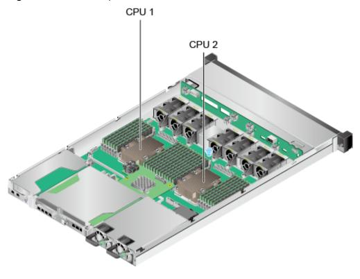
Figure 5-13 Processor positions
