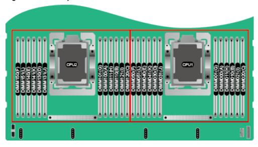
Figure 5-20 DCPMM and DDR4 memory configuration guidelines (1 processor)
