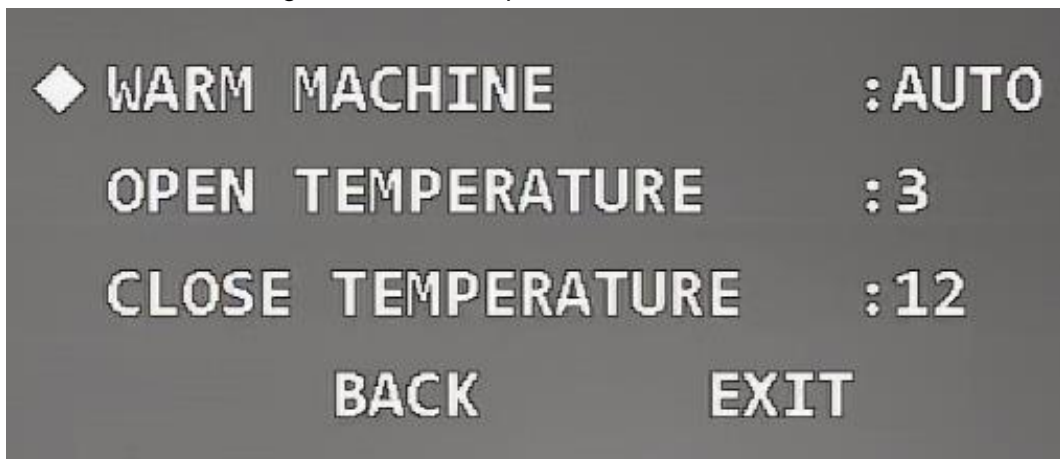
Figure 3-70 Set temperature control
