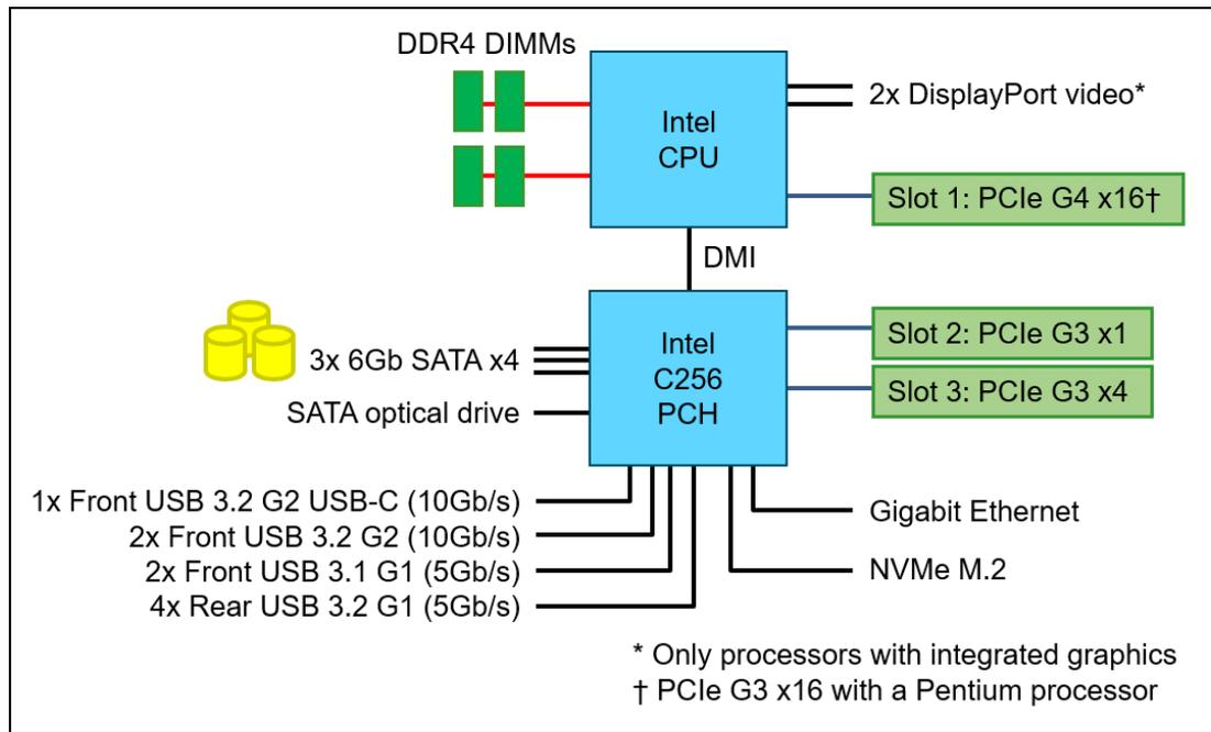
Figure 5. ST50 V2 system architectural block diagram
