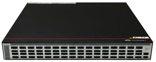
The CloudEngine 8850E-32CQ-EI series switch provides 32 x 100GE QSFP28 ports and one 10GE SFP+ port. The following figure shows the switch appearance.
