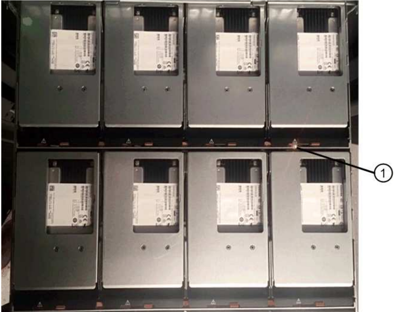
(1) Attention LED light on for the drive on the top right side
