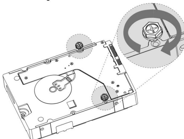
Step 3 Align the two screws with the holes on the device.
