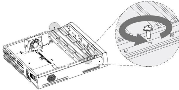
**Step 4** Align the four screw holes on the disk to those on the drive bracket and fix the disk on the bracket.
