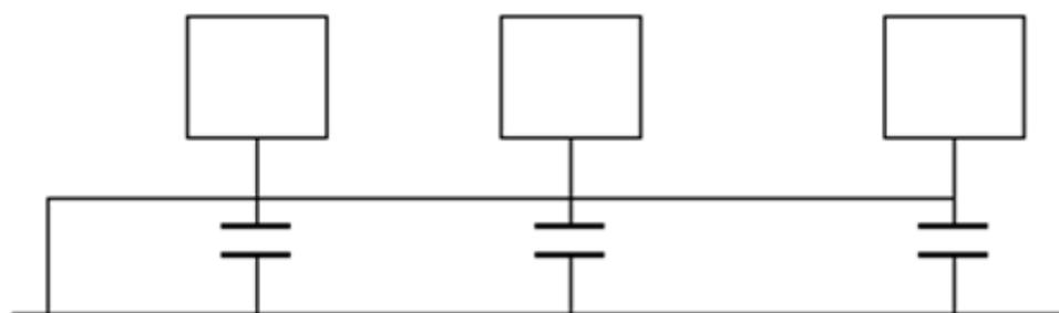
When connecting devices of huge size (the device physical dimension and connection cable is big comparing with the wave path of existed interference), then there is possibility of interference when the current goes through the chassis and cable. In this situation, the interference circuit path usually lies in the system ground circuit.
