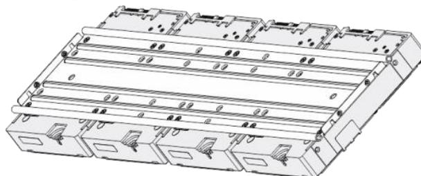
Step 6 Place the bracket to the device and then fasten the screws on the sides of the bracket.
