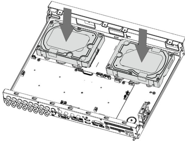
**Step 4** Turn the device and put in the other two screws, and then fasten all screws to fix the HDD to the device.
