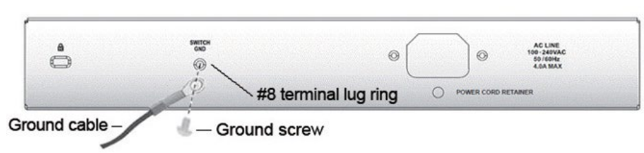
Figure 2.10 – Connect a Grounding Cable
