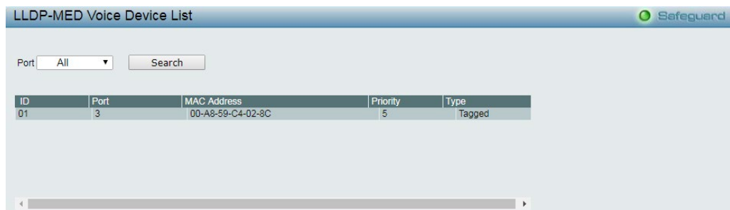
Figure 4.56 - Configuration > Voice VLAN > LLDP-MED Voice Device List
