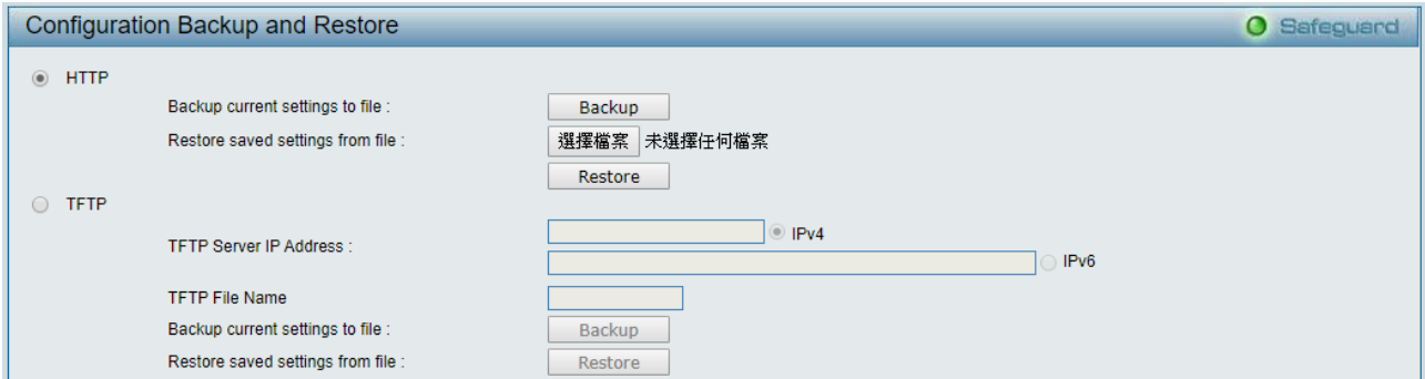
Figure 4.8 – Tool Menu > Configure Backup and Restore
