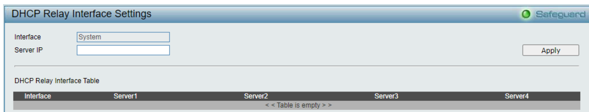
Figure 4.82 - Configuration > DHCP Relay > DHCP Relay Interface Settings
