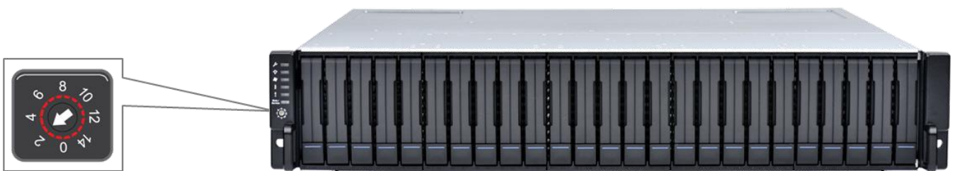
Figure9: Expansion enclosure ID
