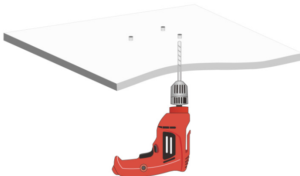
Figure 2-10 Drilling holes in the ceiling tile
