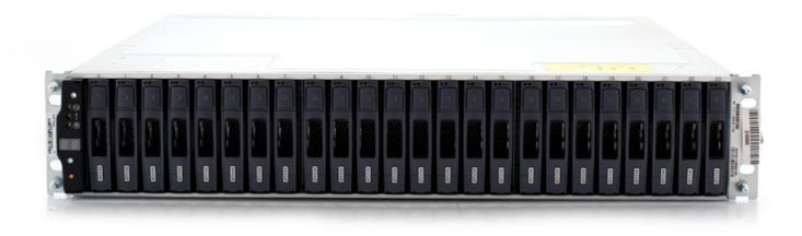
The front of the device is simple enough with a NetApp-branded bezel covering the drive bays. On the left-hand side is the power button, along with an LED display indicating faults and activity status.
