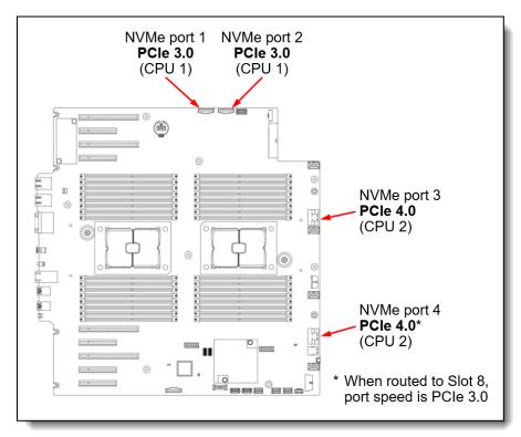
Figure 8. Onboard NVMe port speeds
