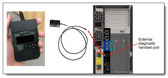
Figure 12. ST650 V2 External Diagnostics Handset
