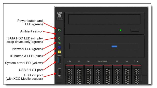
Figure 11. ST650 V2 front operator panel
