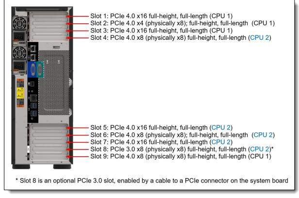
Figure 10. ST650 V2 PCIe slots
