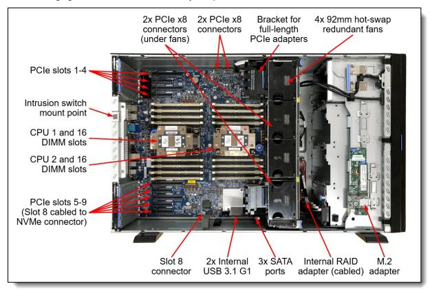
The following figure shows the locations of key components inside the server.
