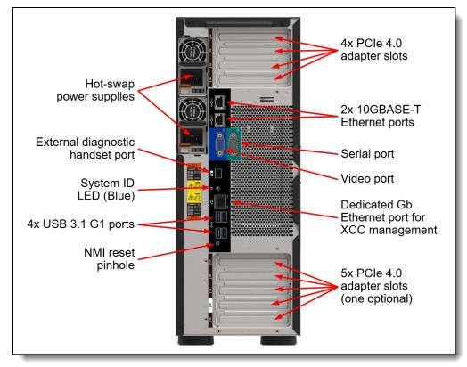
The following figure shows the components visible from the rear of the server.
