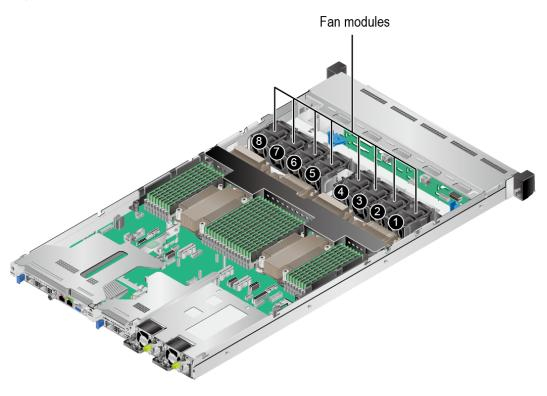
Figure 5-32 Positions of the fan modules
