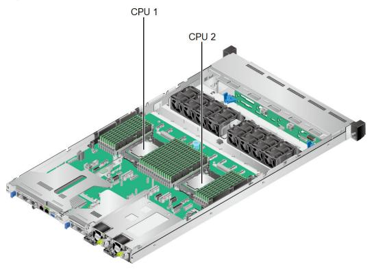
Figure 5-13 Positions of the processors
