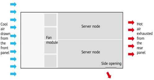
Figure 3-1 Top view of the X6000 V6 air flow
