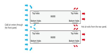
Figure 3-2 Side view of the X6000 V6 air flow
