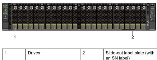
Figure 5-2 Front panel of a server with 24 x 2.5" drives
