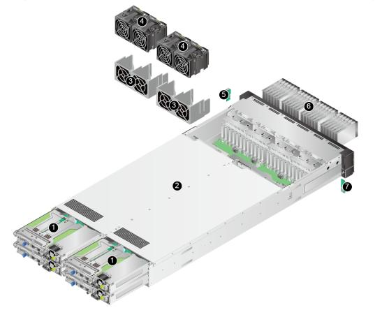
Figure 4-1 Physical structure of an X6000 V6 server with 24 x 2.5" drives (example)
