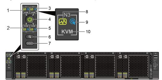
Figure 5-3 Indicators and buttons on the front panel
