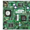
BMB-CMM-002 Mini CMM Installs in SBM-XEM-002M, SBM-IBS-Q3616M, SBM-IBS-Q3618M SBM-XEM-X10SM, SBM-IBS-F3616M and SBM-XEM-F8X4SM CMM (Chassis Management Module)
