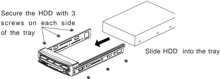
5. Once the HDD is securely placed into the SCA tray, you can install the SCA drive tray back to the chassis.
