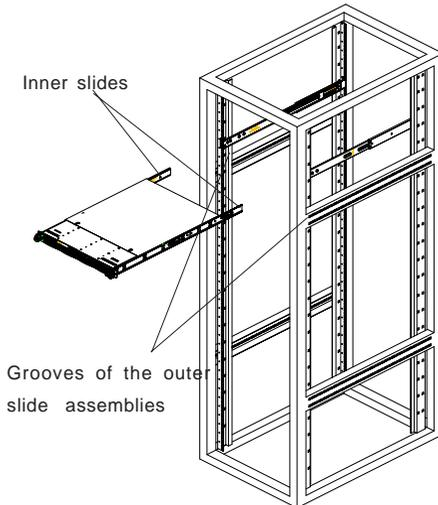
2. Push the chassis all the way to the back of the outer slide assemblies as shown below: (The plastic bezel is not included in the package.)
