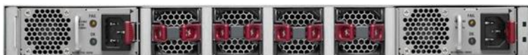
Figure 6. Cisco Nexus 3548-X and 3524-X with red handles indicating port-side intake airflow
