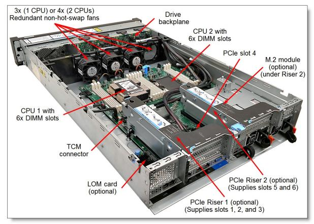
Figure 6. Internal view of the SR550
