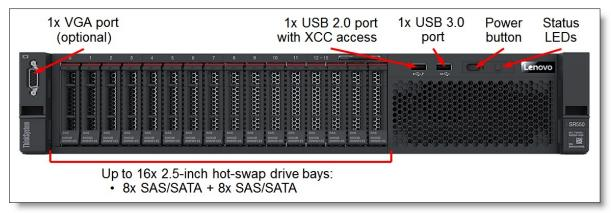
Figure 4. Front view of the SR550: Up to 16x 2.5-inch drive bays
