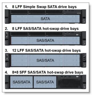
Figure 7. Internal drive bay configurations
