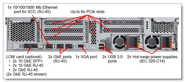
Figure 5. Rear view of the SR550
