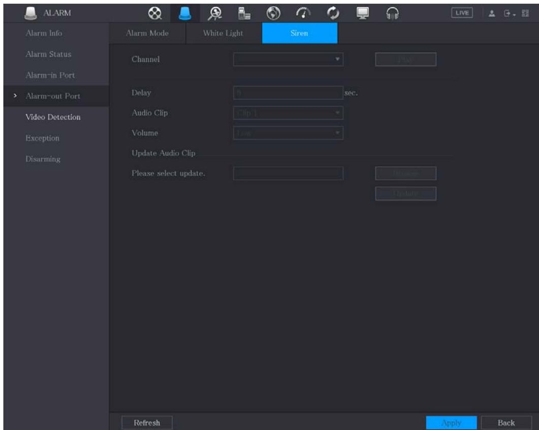
**Step 2** Configure the settings for the siren parameters.
