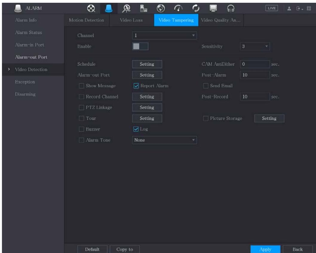
**Step 2** To configure the settings for the tampering detection parameters, see “5.10.4.1 Configuring Motion Detection Settings.”
