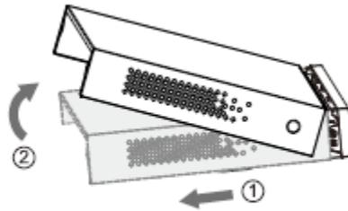
Step 3 Turn over the device, and align the HDD to the four holes of bottom panel, and then fix the HDD with screws.
