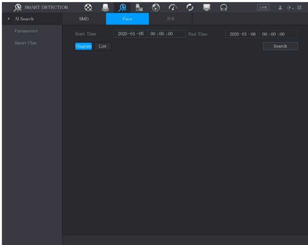
**Step 2** In the **Start Time** box and **End Time** box, enter the time.
