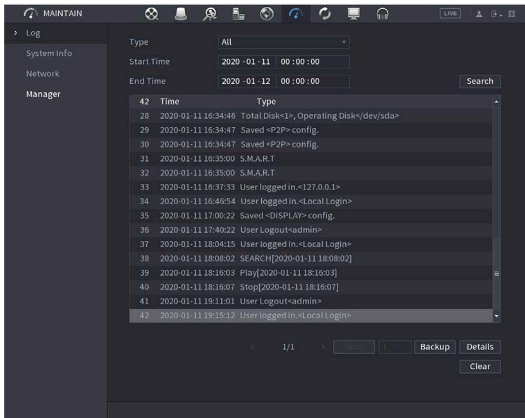
**Step 2** In the **Type** list, select the log type that you want to view (**System, Config, Storage, Record, Account, Clear Log, Playback, and Connection**) or select **All** to view all logs.
