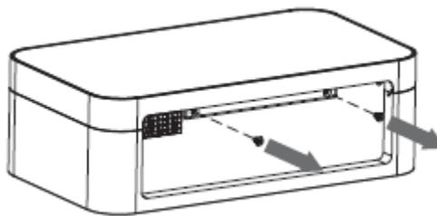
Step 2 Remove the screws to take off the bracket.
