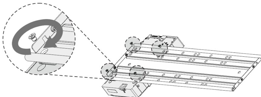
**Step 5** Fix other disks on the bracket as needed.
