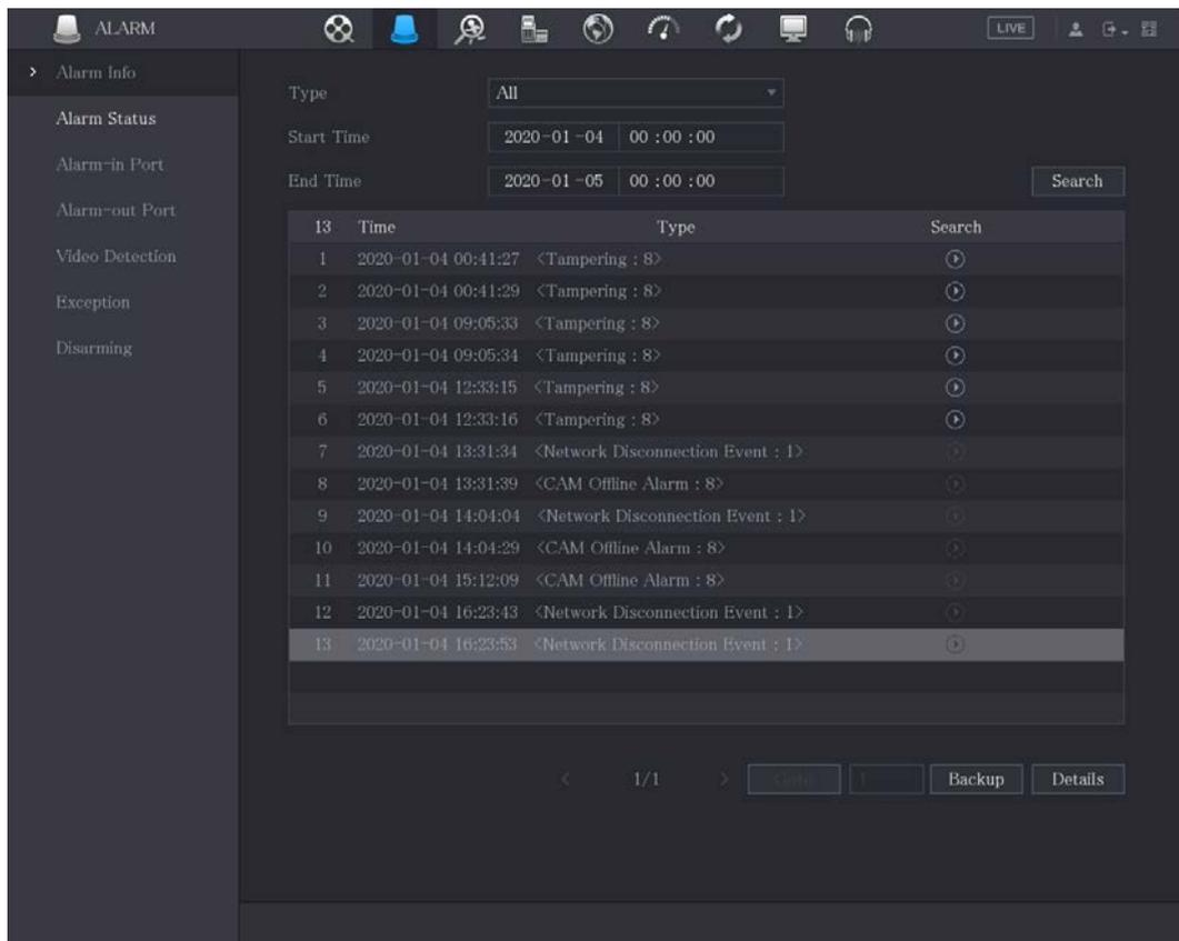
**Step 2** In the **Type** list, select the event type; In the **Start Time** box and **End Time** box, enter the specific time.
