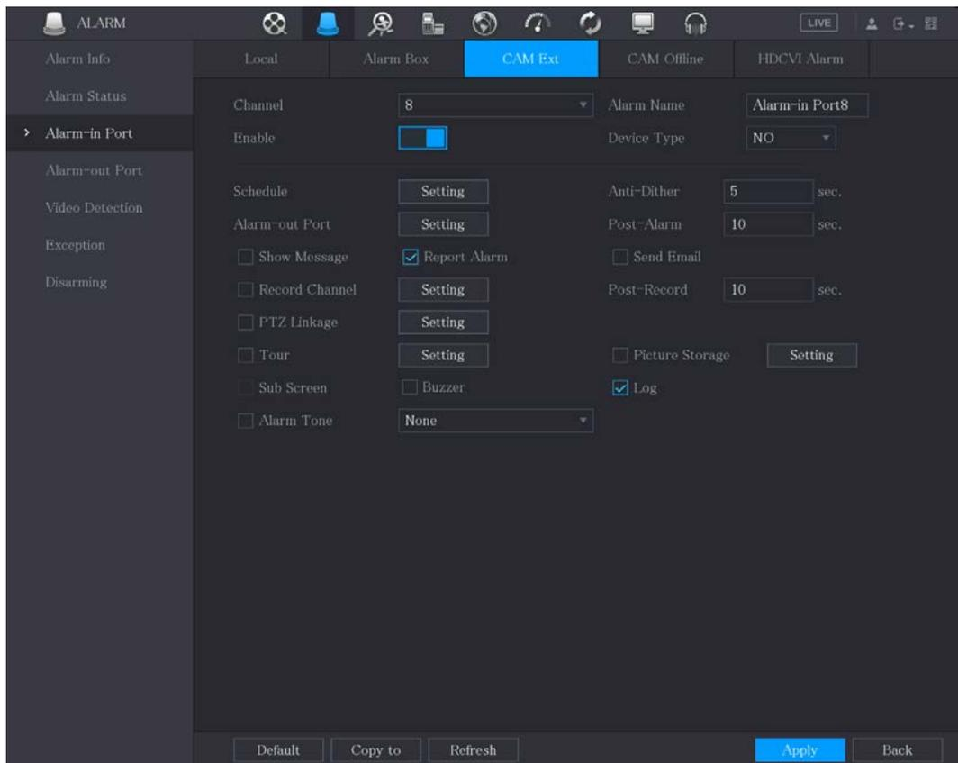
**Step 2** Configure the alarm input settings from the external IPC. For details, see Table 5-36.
