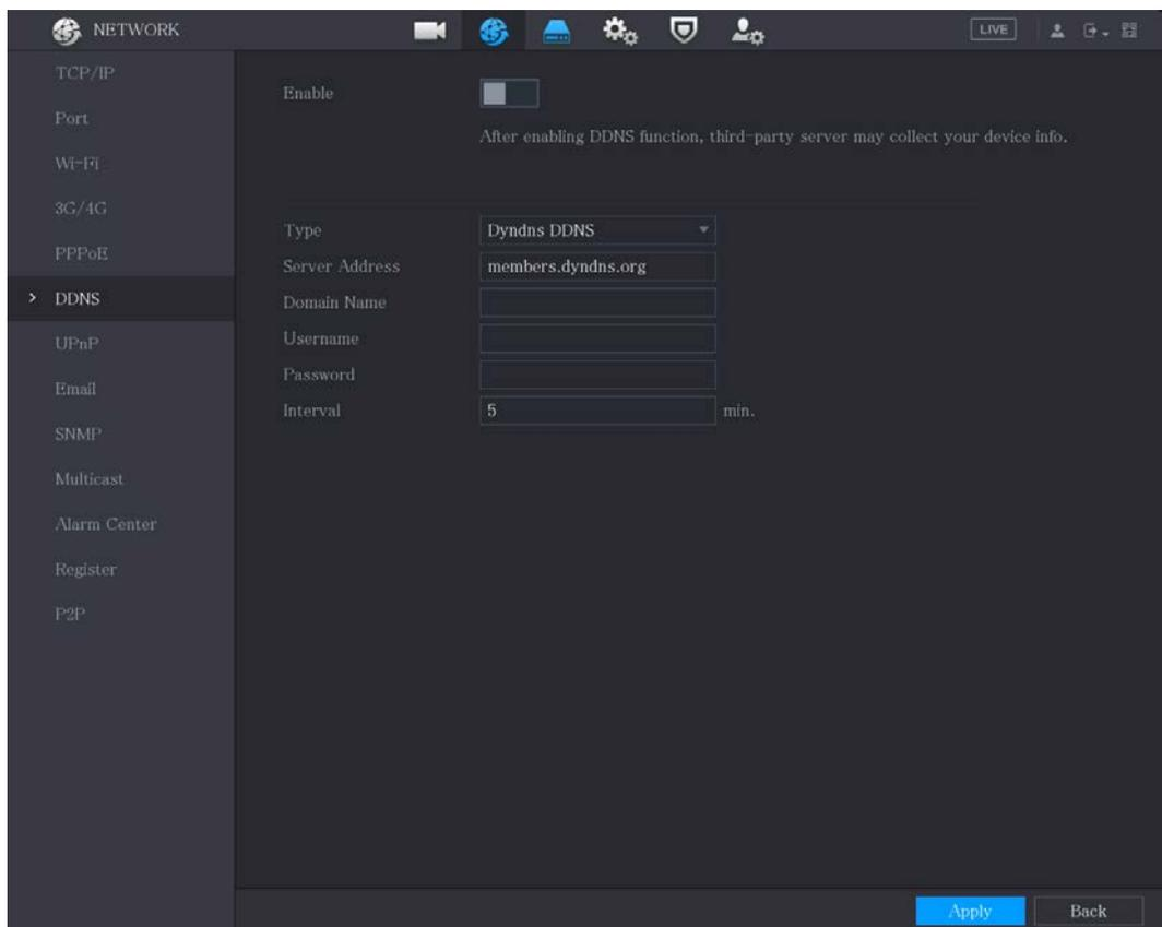
**Step 2** Configure the settings for the DDNS parameters.
