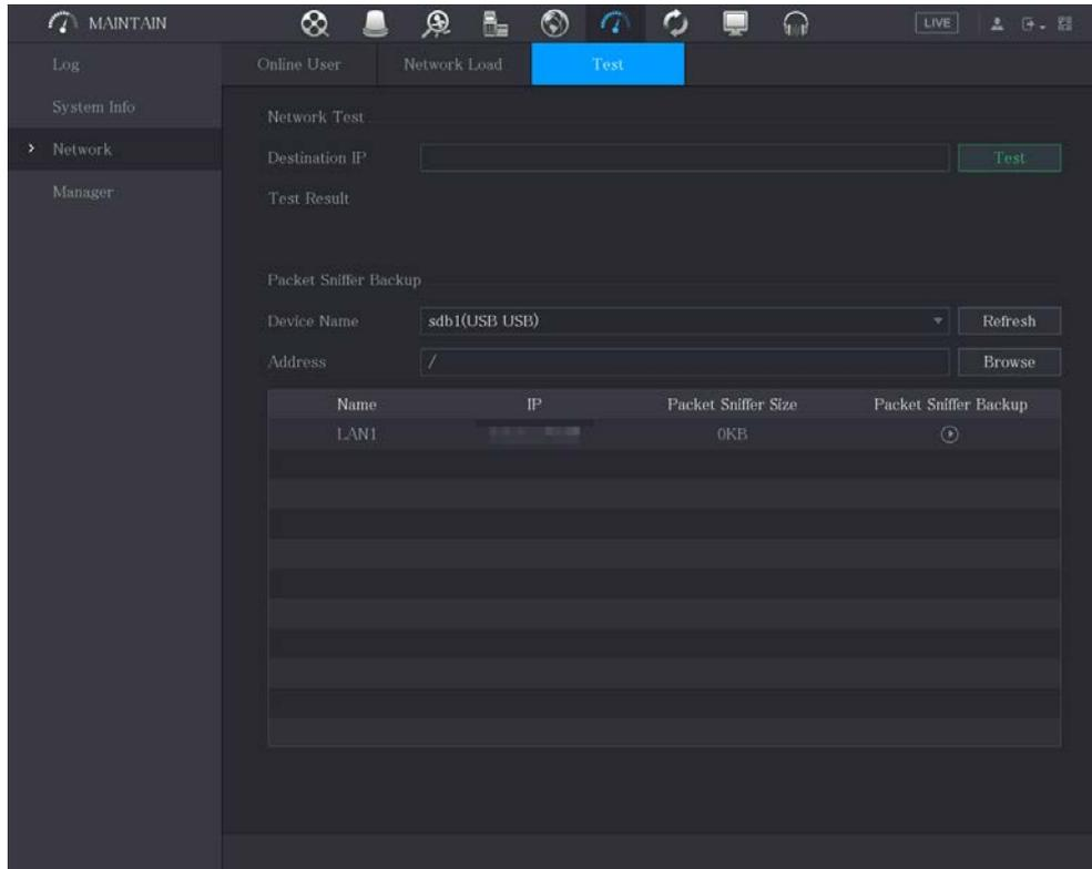
**Step 2** In the **Destination IP** box, enter the IP address.
