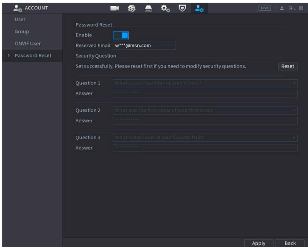
**Step 2** Enable the Password Reset function.
