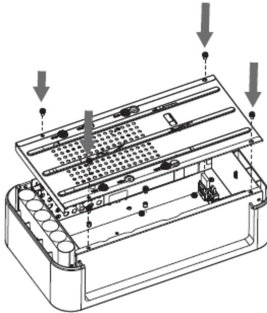
**Step 5** Put back the cover and then fasten the screws.
