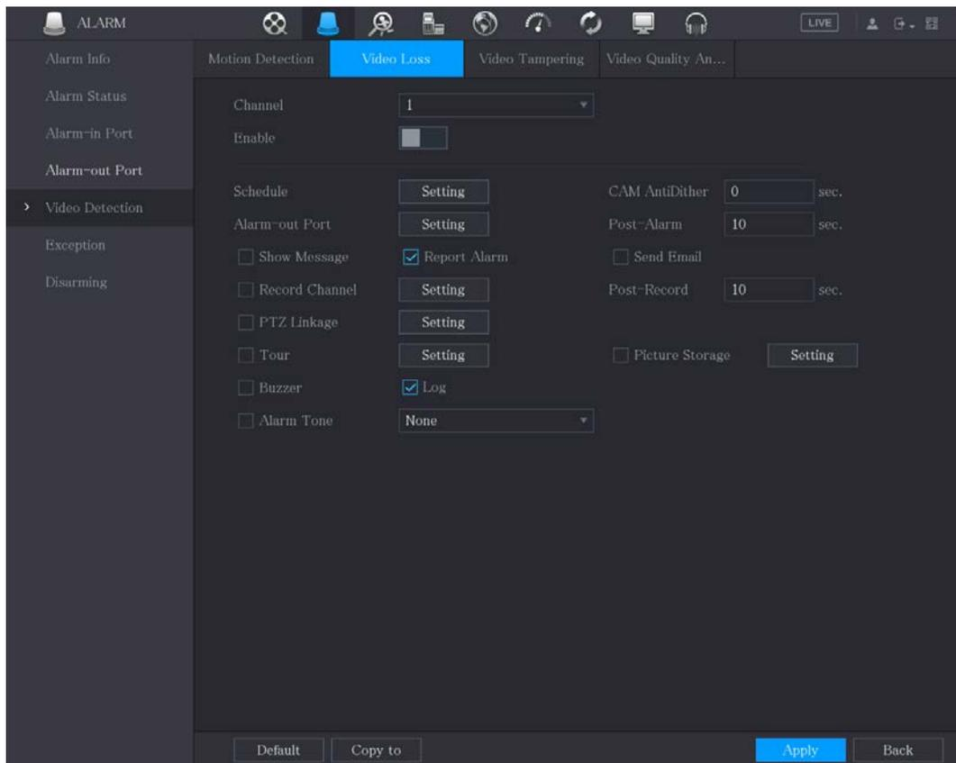
**Step 2** To configure the settings for the video loss detection parameters, see “5.10.4.1 Configuring Motion Detection Settings.”
