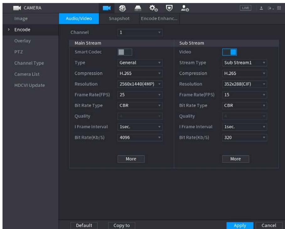
**Step 2** Configure the settings for the main/sub streams parameters.
