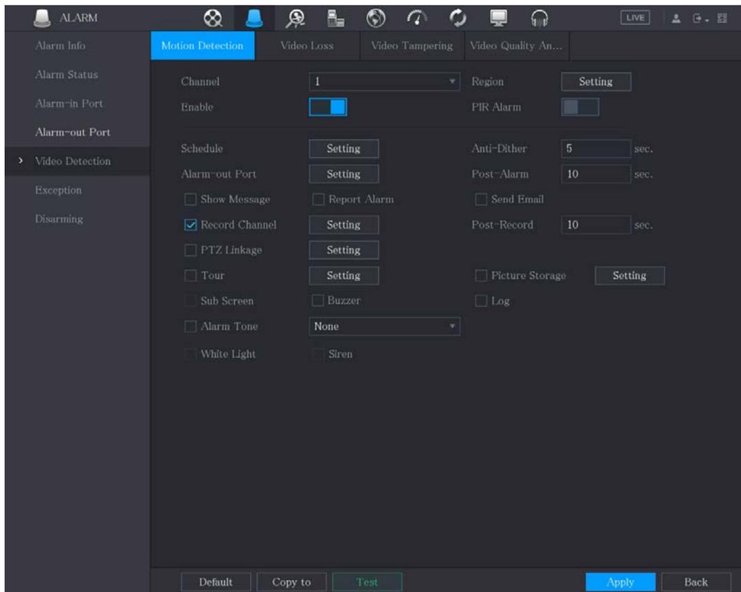
**Step 2** Configure the settings for the motion detection parameters.
