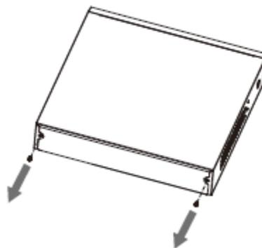
**Step 2** Remove the cover in the direction of the arrow as shown in the figure below.
