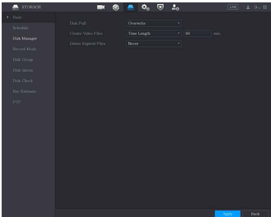
**Step 2** Configure the settings for the basic settings parameters.
