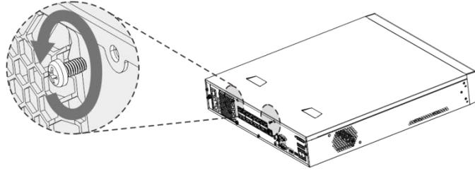
**Step 2** Remove the cover along the direction shown in the following arrow.
