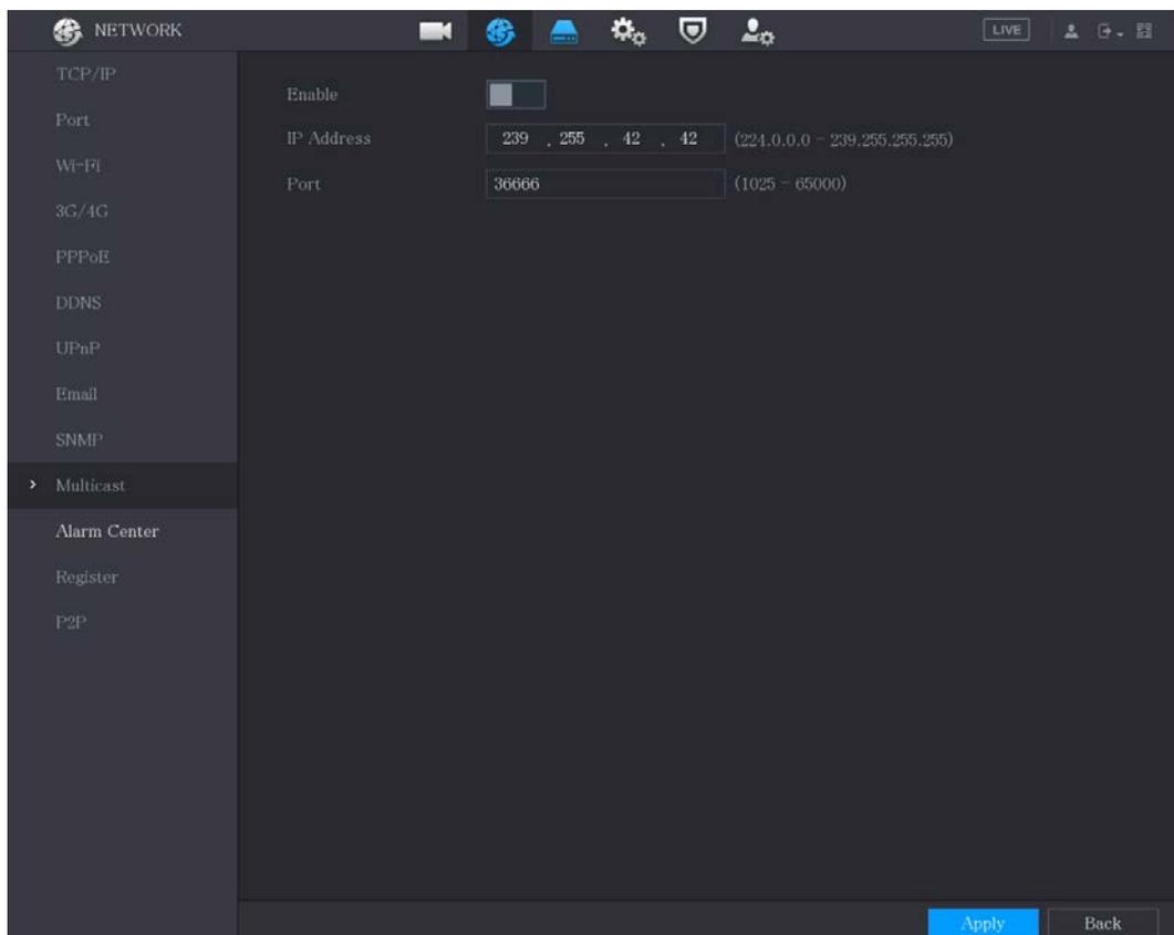
**Step 2** Configure the settings for the multicast parameters.
