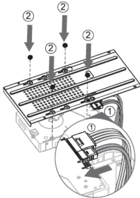
Figure 2-11 Connect cables
