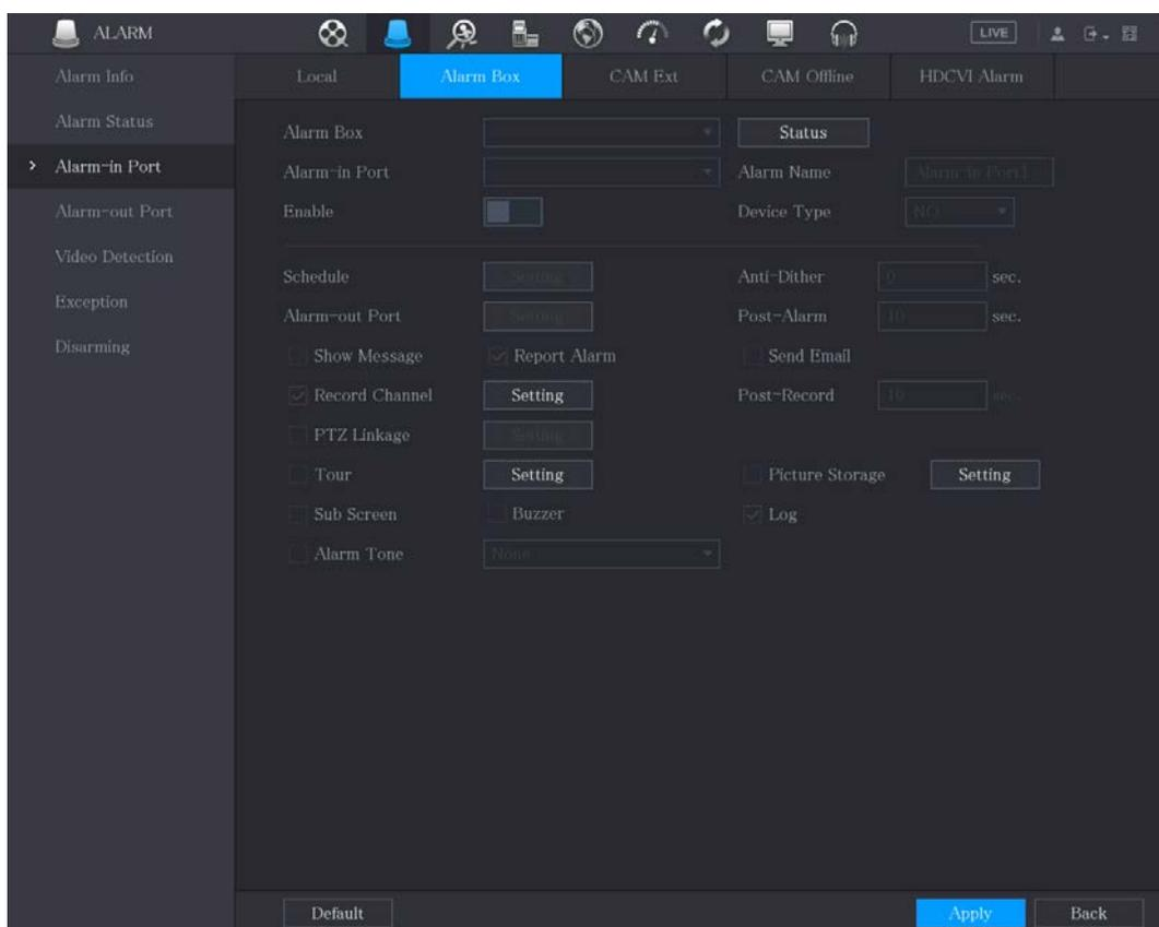
**Step 2** In the **Alarm Box** list, select the alarm box number corresponding to the address number configured by the DIP switch on the Alarm Box.
