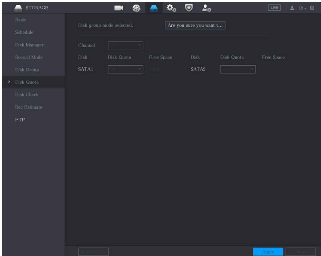
**Step 2** Select the channels you want to configure, and select quota from the drop-down list of corresponding HDD.
