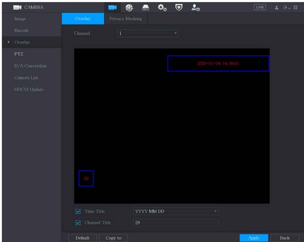
**Step 2** Configure the settings for the text overlay parameters.
