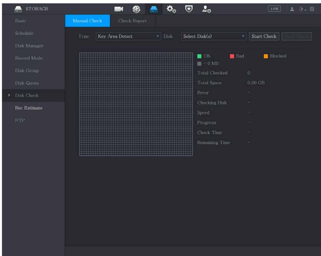
**Step 2** In the **Type** list, select **Key Area Detect** or **Global Check**; and in the **Disk** list, select the HDD that you want to detect.
