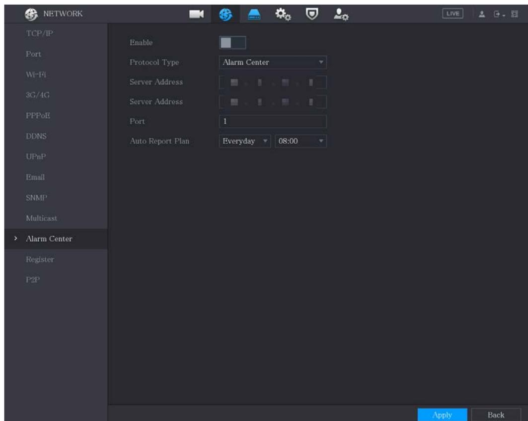
**Step 2** Configure the settings for the alarm center parameters.
