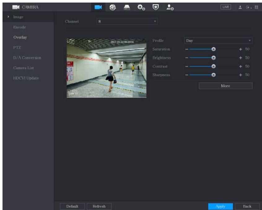
**Step 2** Configure the settings for the image parameters.
