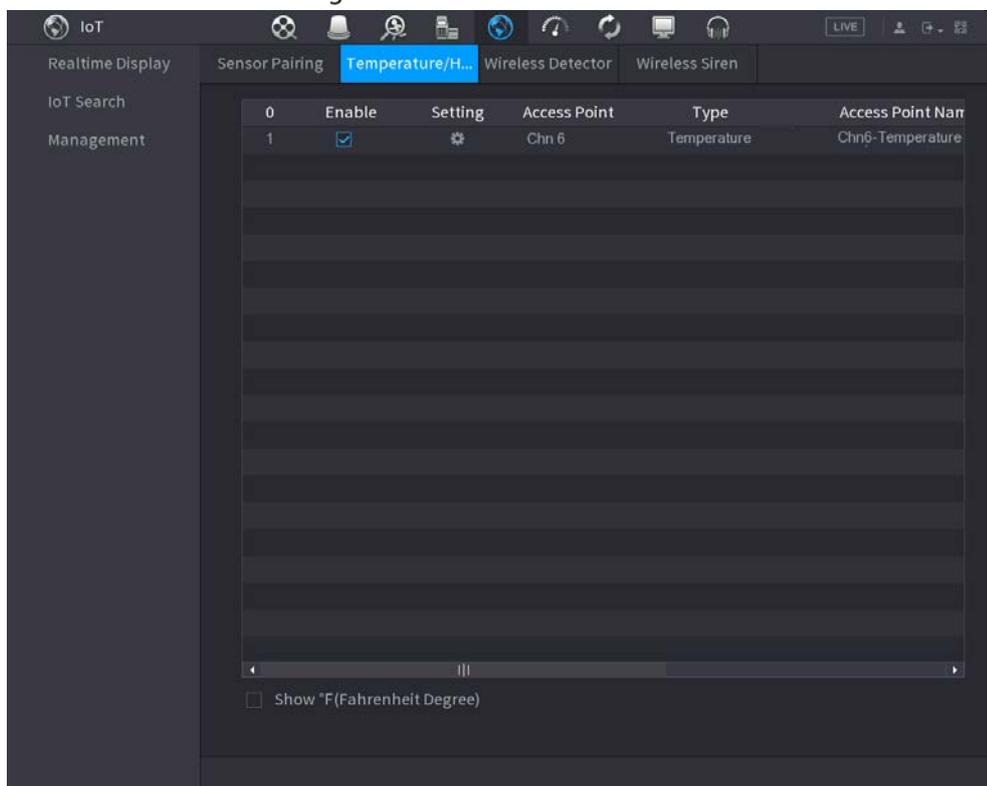
The Device starts detecting the temperature and humidity data from the camera and display on the **Realtime Display** interface.
