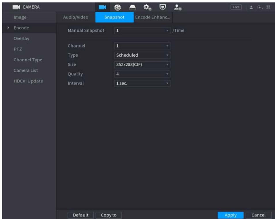
**Step 2** Configure the settings for the snapshot parameters.
