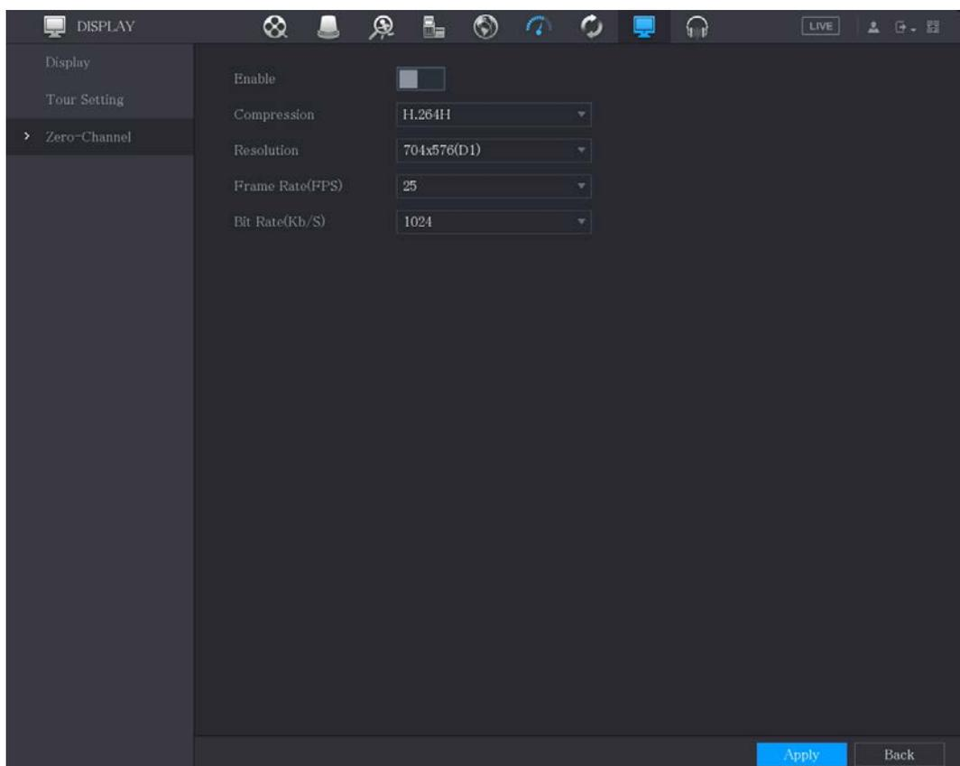
**Step 2** Configure the settings for the zero-channel parameters.
