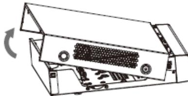
**Step 3** Turn over the device, and align the HDD to the four holes of bottom panel, and then fix the HDD with screws.
