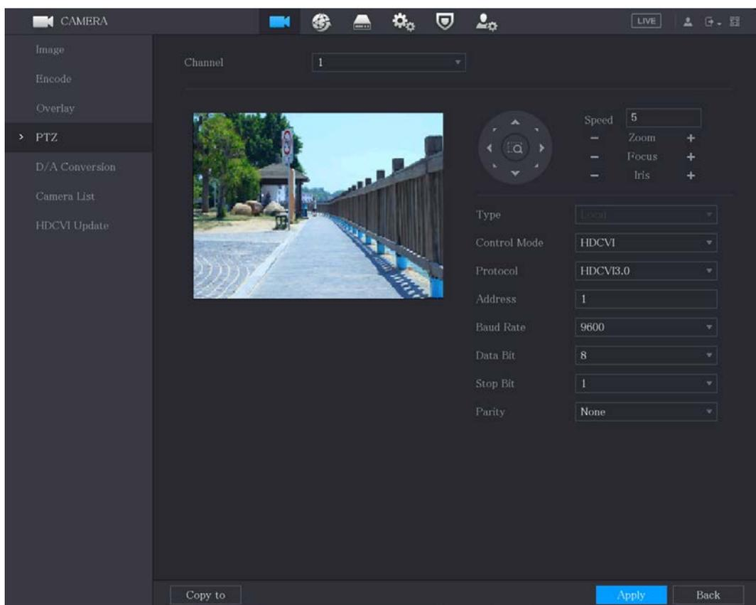
**Step 2** Configure the settings for the PTZ connection parameters.
