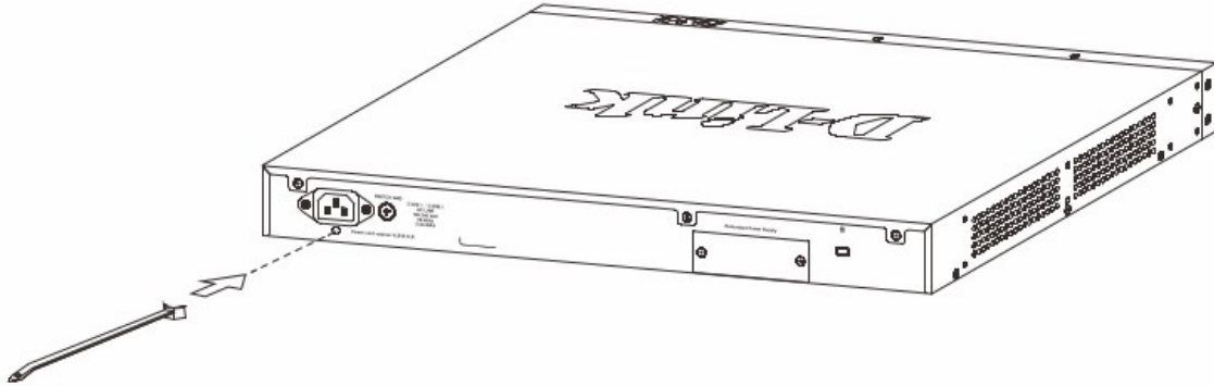
Figure 8 — Insert tie wrap into the switch
