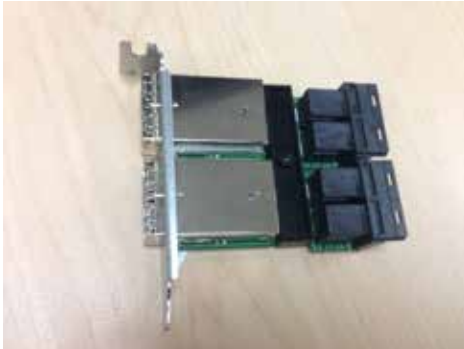
Figure 3EL-17. Mini-SAS HD Internal to External Adapter
