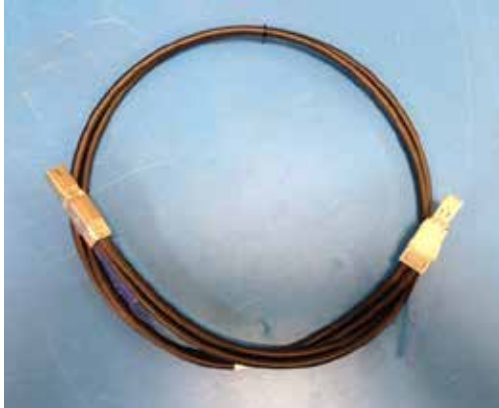
Figure 3EL-16. External Mini-SAS HD to External Mini-SAS HD Cable
