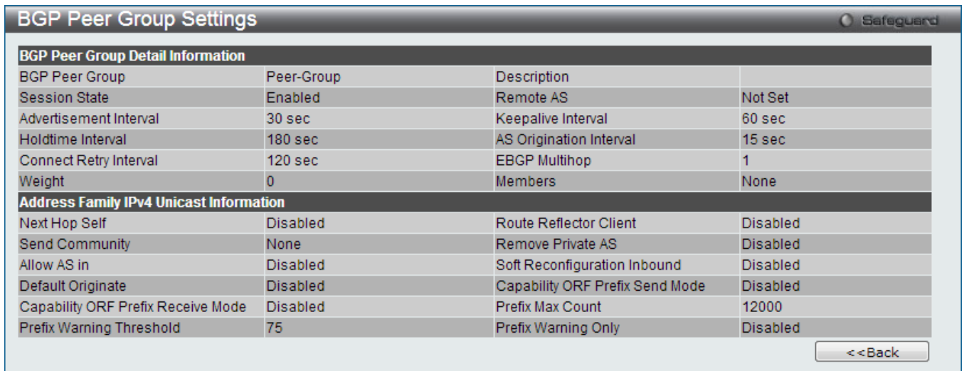
Figure 6-147 BGP Peer Group Settings - View Detail window
