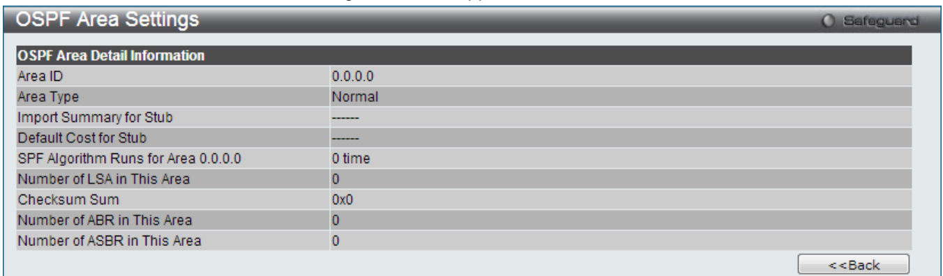
Figure 6-45 OSPF Area Settings - View Detail window
