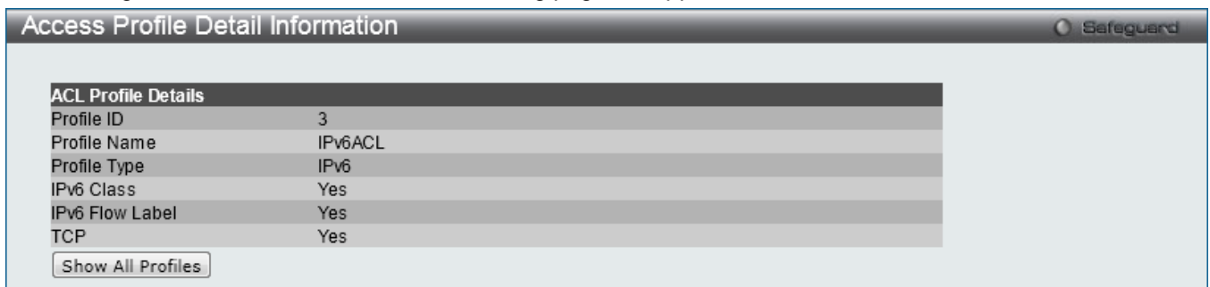
Figure 8-14 Access Profile Detail Information window (IPv6 ACL)
