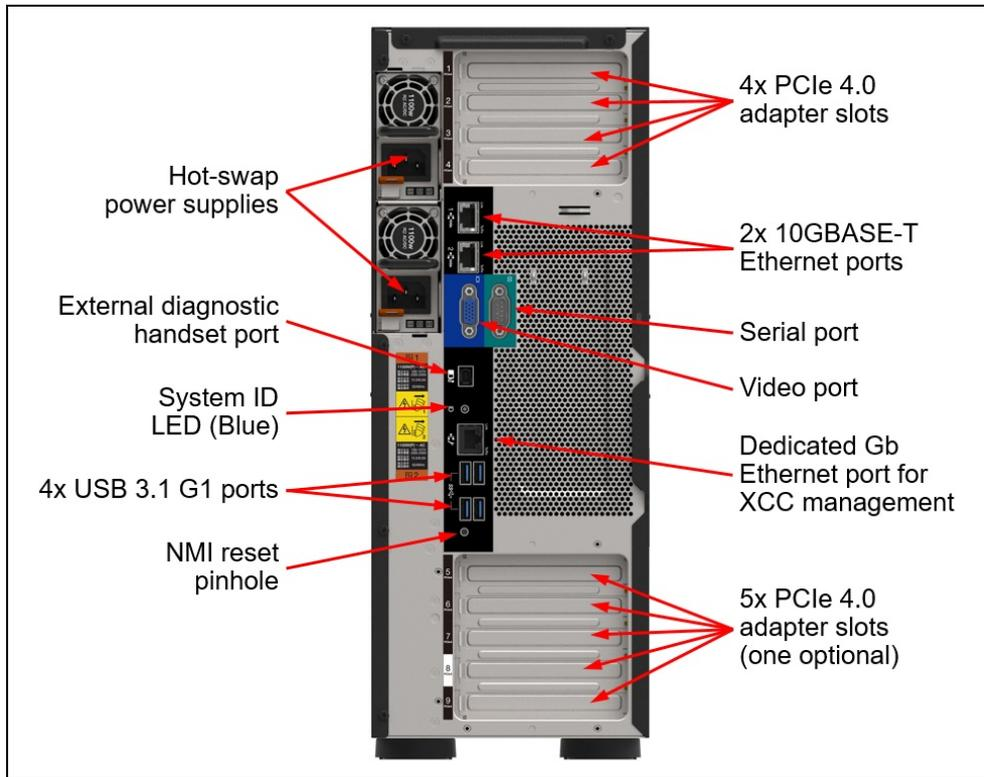
Figure 4. Rear view of the ThinkSystem ST650 V2
