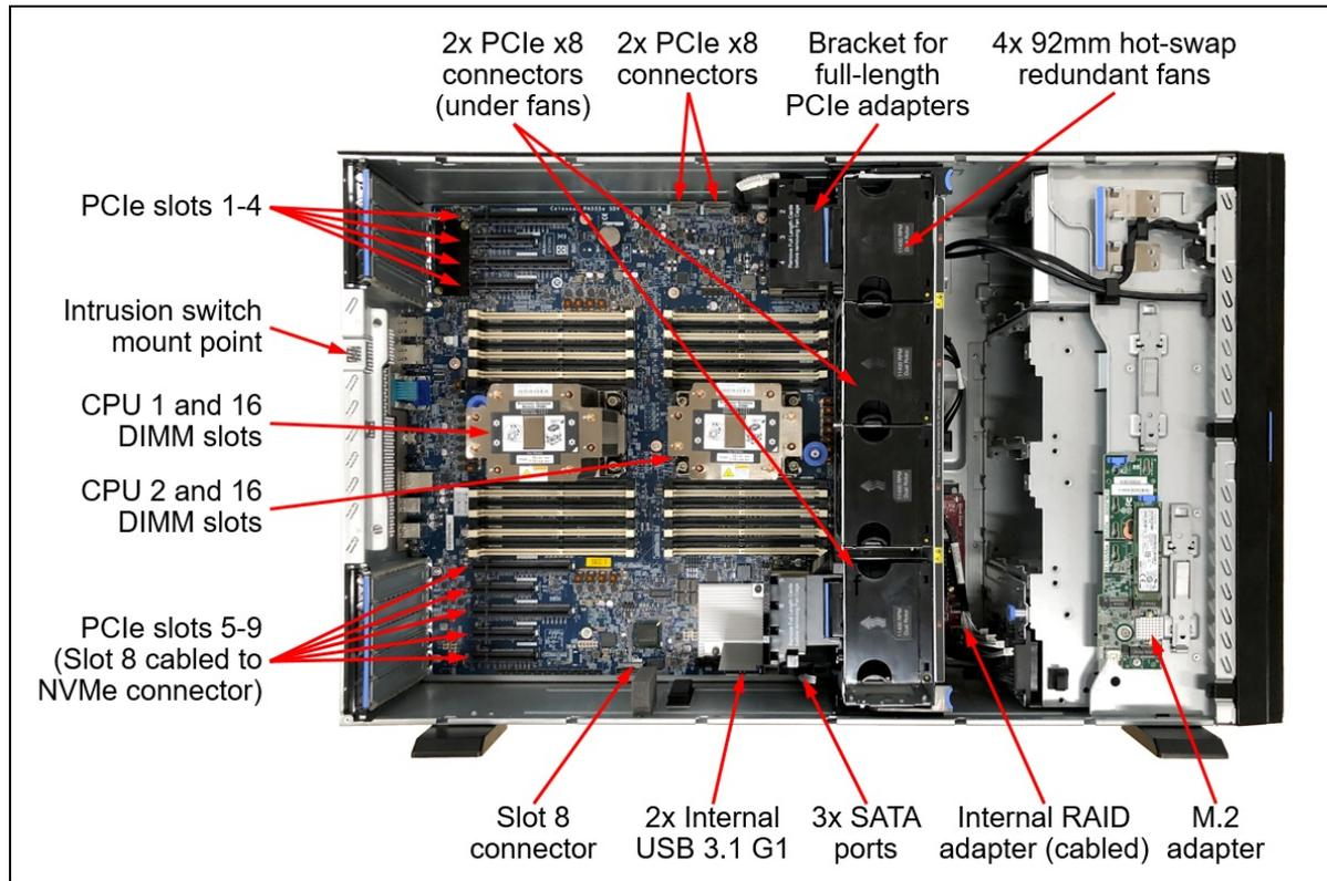
Figure 5. Internal view of the ThinkSystem ST650 V2
