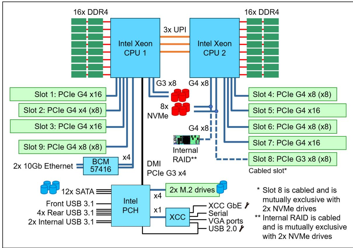
Figure 6. ST650 V2 system architectural block diagram
