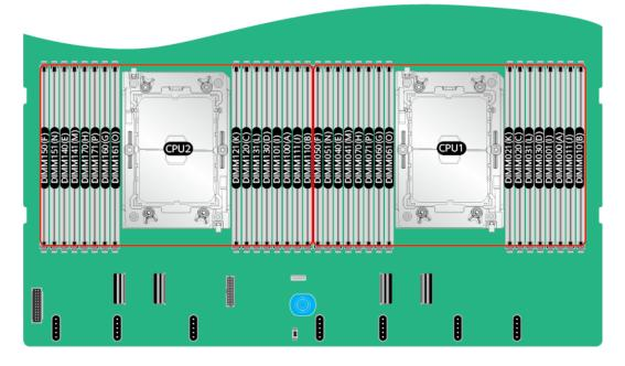
Figure 5-16 DDR4 memory module installation guidelines (1 processor)
