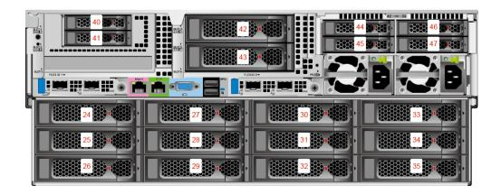
**Figure 5-14** Drive numbering (I/O module 1 configured with 3.5" drives + I/O module 2 configured with 2.5" drives + I/O module 3 configured with NVMe drives)
