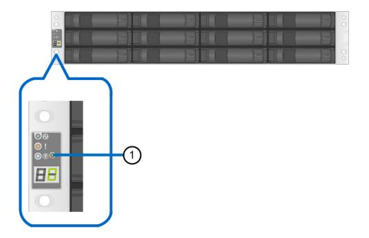
The following figure shows the ODP push button on the E2824 and E5724 controller shelf and the DE224C drive shelf.
