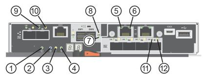
E5700 controller with quad-port SFP (FC) host interface card
