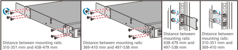
**Step 3** Install four floating nuts on the front mounting rails, two on each side.
