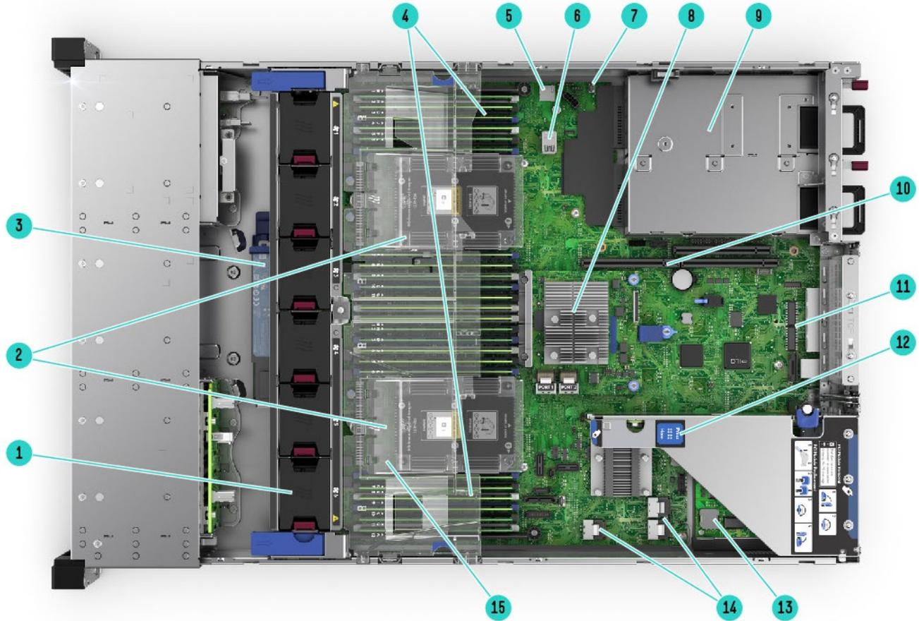
Internal View 8SFF chassis – with optional 2<sup>nd</sup> CPU, FlexLOM, Smart array shown
