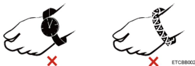
Figure 8-2 Removing conductive objects
