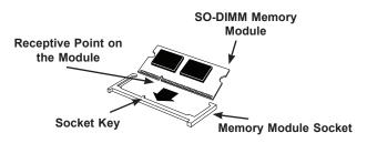
2. Line up the bottom of the SO-DIMM memory module with the edge of the horizontal socket
