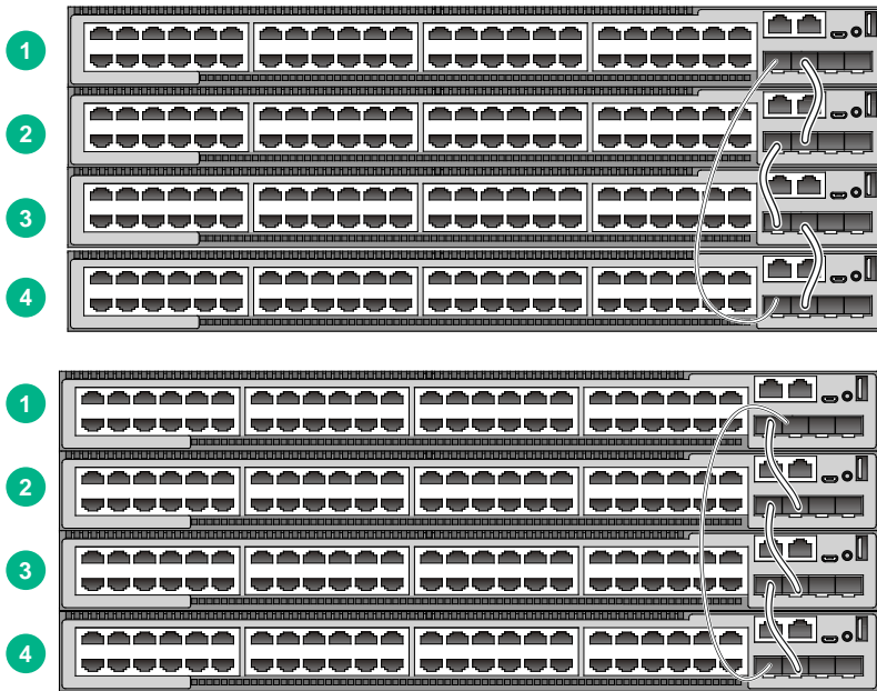
Figure 4-4 Connecting the switches in one rack
