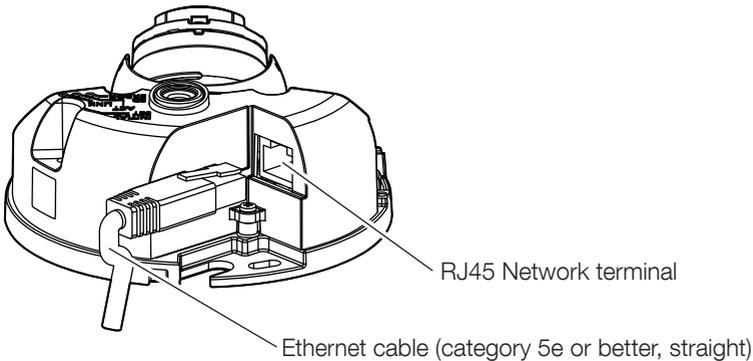
Connect an Ethernet cable (category 5e or better, straight) to the RJ45 Network cable or RJ45 Network terminal.
