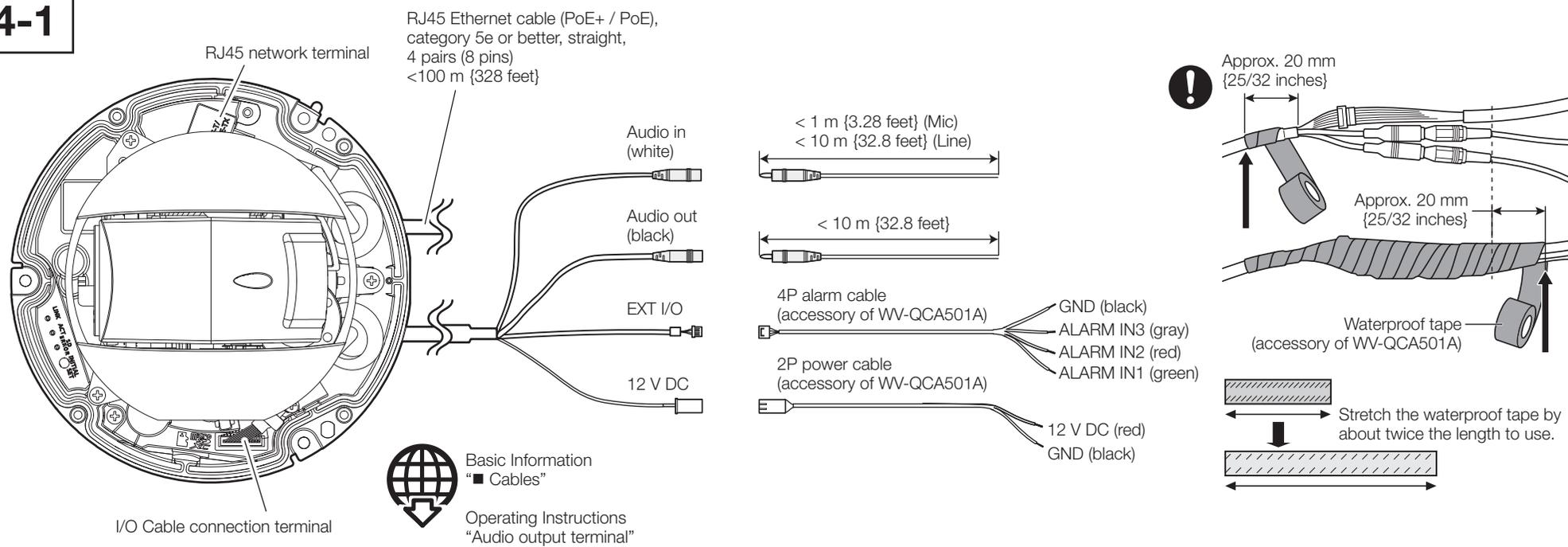
■ When connecting the RJ45 Ethernet cable (locally procured) directly to the camera.
