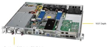
Front-Access DC Redundant PSU (Default)
