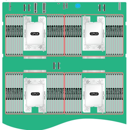
Figure 5-15 Positions of the memory modules
