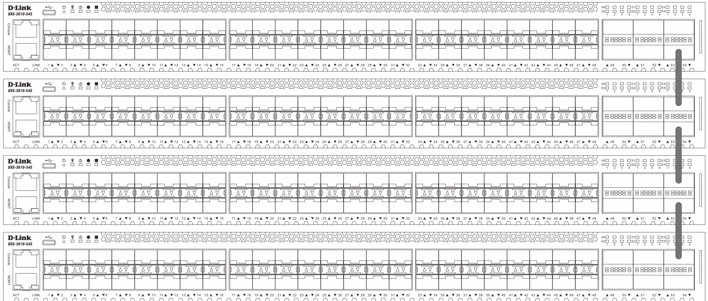
Figure 4-78 Duplex Chain Stacking Topology
