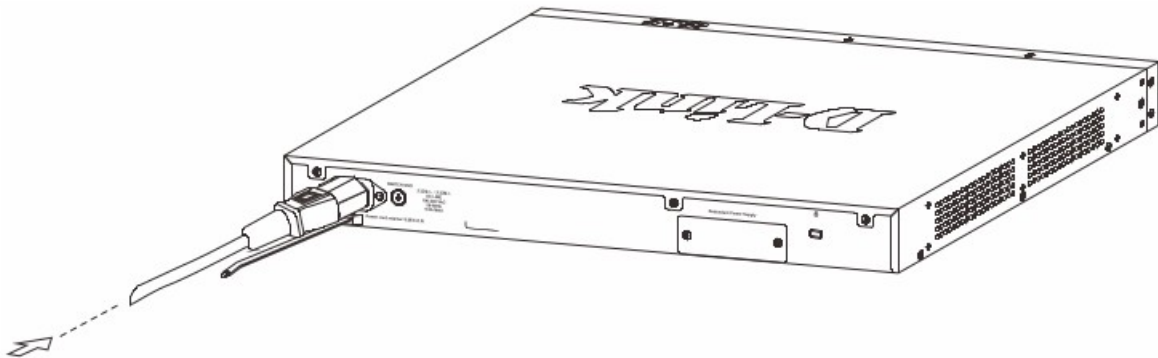
Figure 9 — Connect the power cord to the switch
