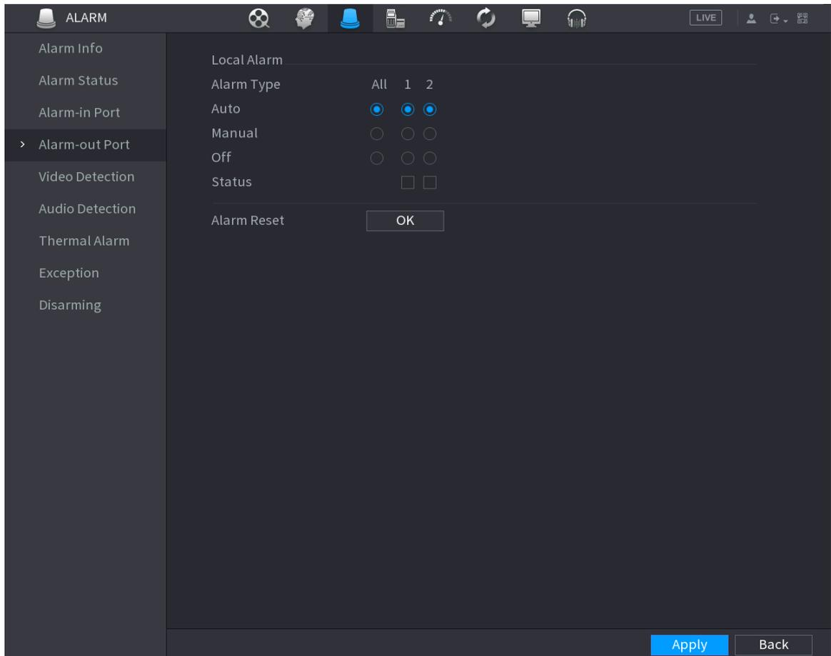
**Step 2** Select the alarm mode of the alarm output channel.
