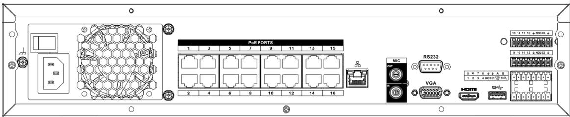
The NVR48-16P-EI series rear panel is shown as below.
