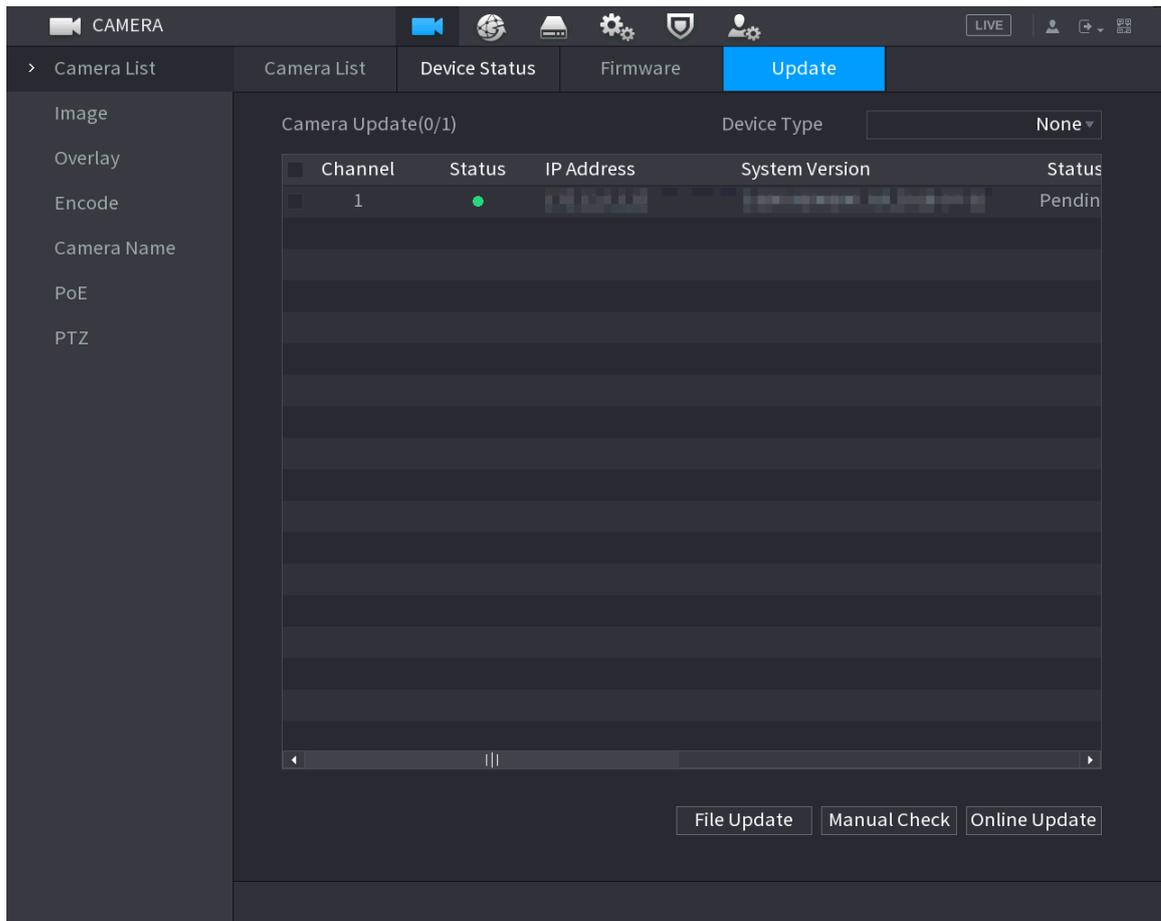
**Step 2** Update the firmware of the connected remote device.
