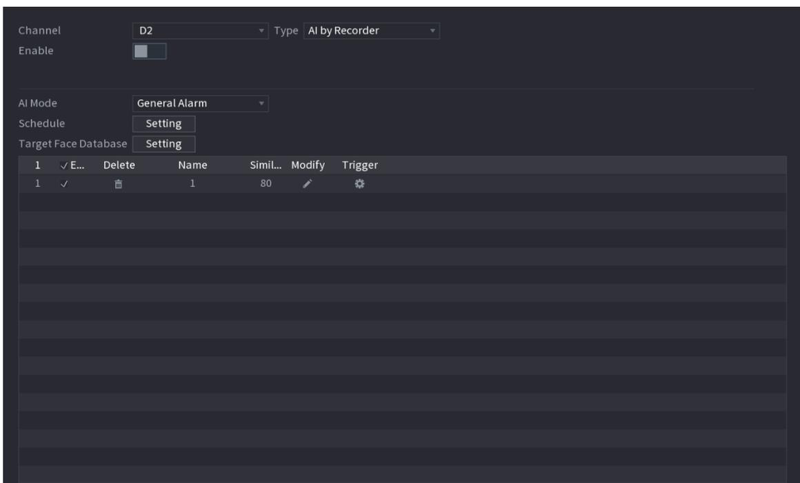
Step 3 Click **Setting** next to **Schedule** to configure arming periods. The corresponding alarm actions are linked by the alarm events triggered during armed period.
