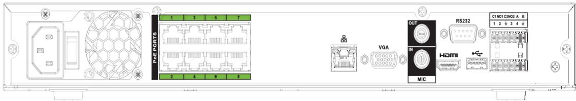
The NVR52-16P-EI series rear panel is shown as below.
