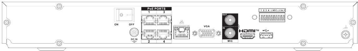
The NVR42-8P-4KS2/NVR42-8P-4KS2/L/NVR42-8P-EI series rear panel is shown as below.
