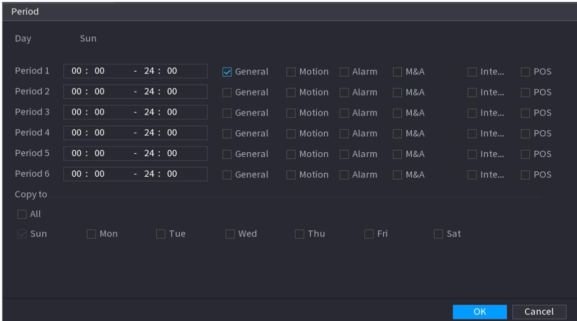
**Step 3** Set one or more recording types from **General**, **Motion** (motion detection), **Alarm**, **M&A** (motion detection and alarm), **Intelligent** and **Alarm**.
