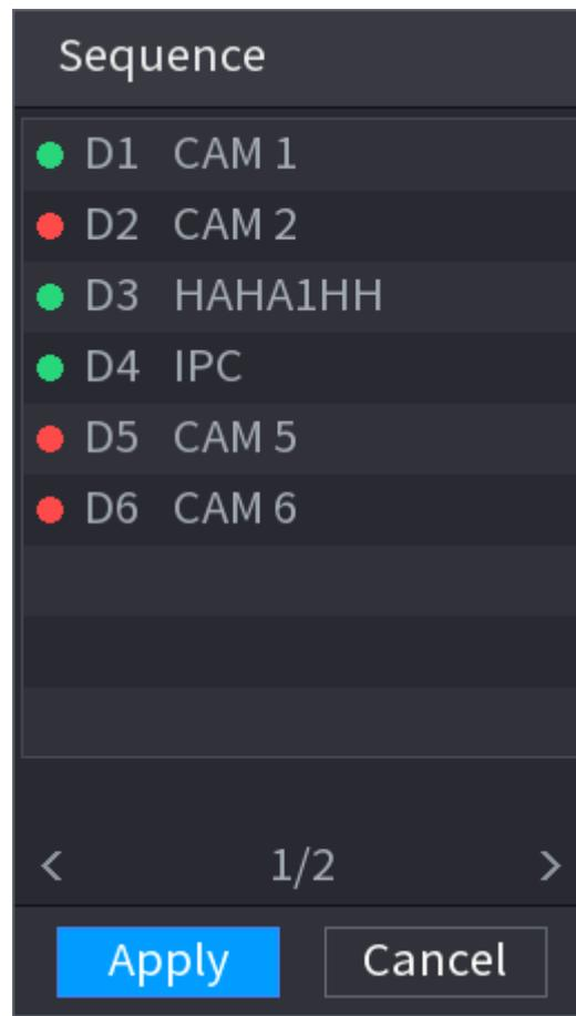
Step 2 On the **Sequence** panel, drag the channel to the desired window, or drag on the live window to switch the position.
