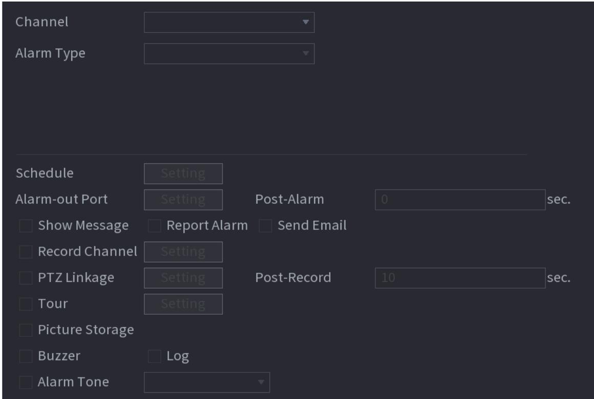
Step 2 Select a channel and set alarm type to heat alarm, and then enable the function.
