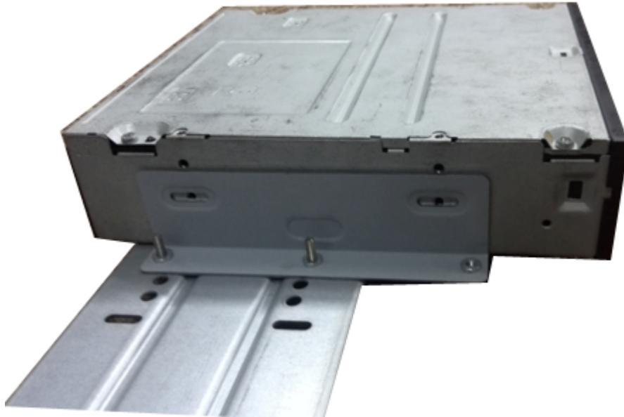
Step 6 Use screw driver to fix the screws.
