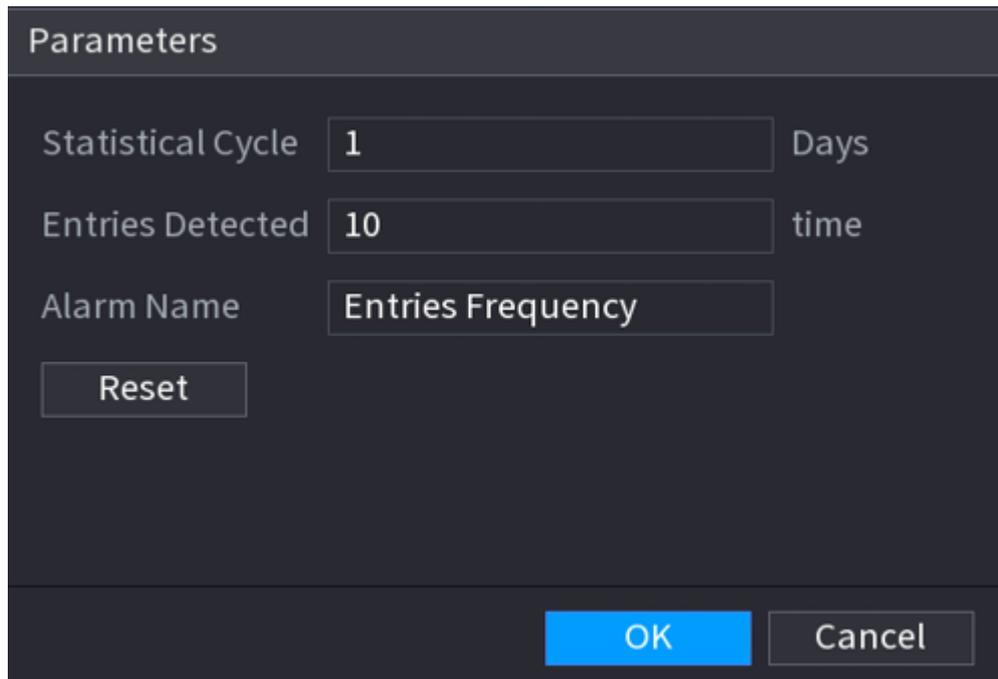
The screenshot shows a dark-themed dialog box titled "Parameters". It contains three input fields: "Statistical Cycle" with the value "1" and the unit "Days", "Entries Detected" with the value "10" and the unit "time", and "Alarm Name" with the value "Entries Frequency". Below these fields is a "Reset" button. At the bottom right of the dialog are "OK" and "Cancel" buttons.
