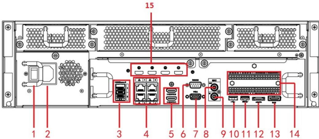
The redundant power series rear panel of NVR616-4KS2 series is shown as below.
