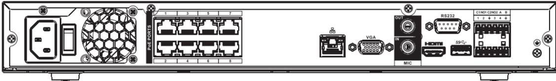
The NVR52-16P-4KS2/NVR42-16P-EI series rear panel is shown as below.
