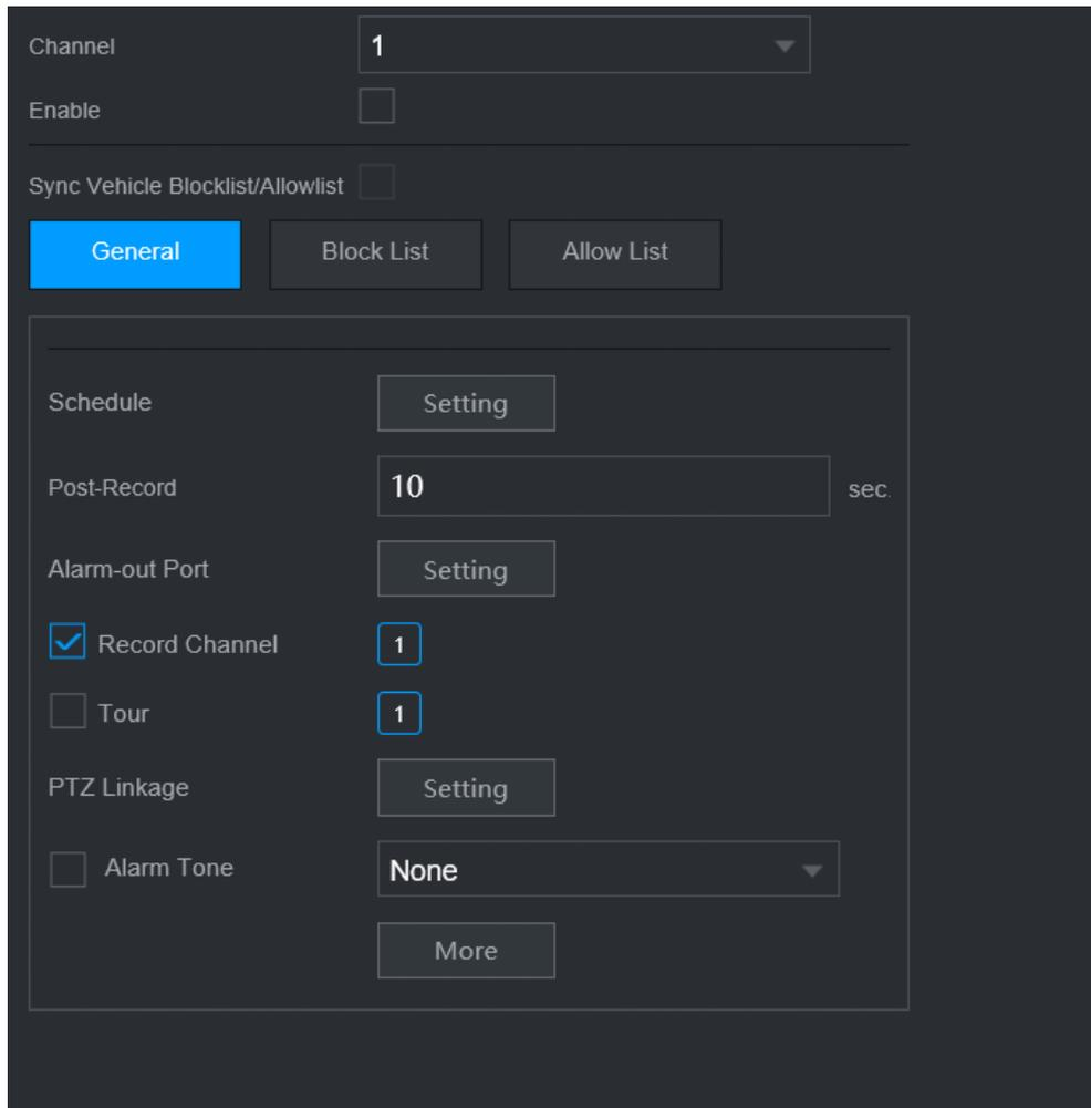
Step 2 Select a channel and then select the **Enable** checkbox to enable ANPR.
