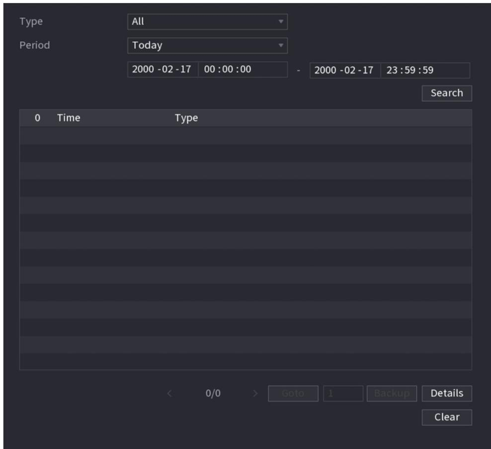
**Step 2** In the **Type** list, select the log type that you want to view (**System, Config, Storage, Record, Account, Clear Log, Playback,** and **Connection**) or select **All** to view all logs.
