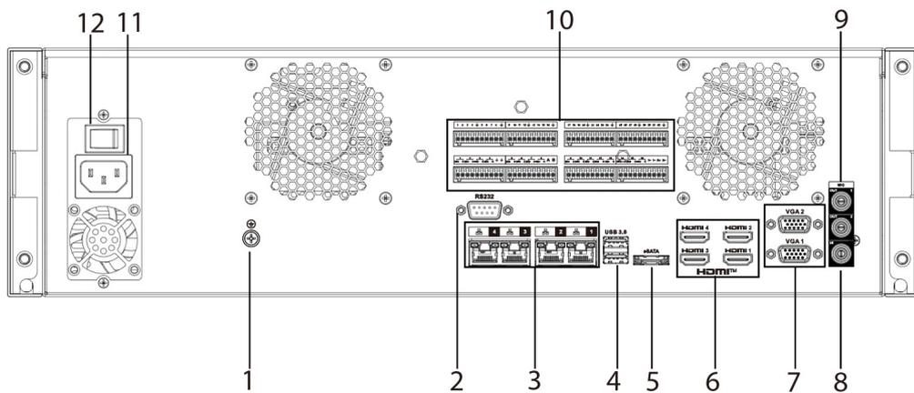
The redundant power series rear panel of NVR616-XI series is shown as below.
