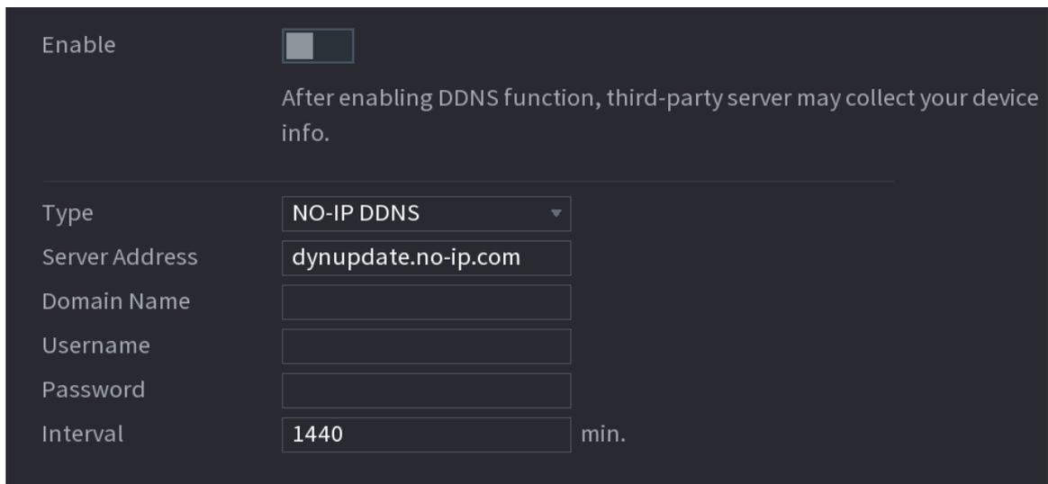
The screenshot shows the DDNS configuration interface. At the top, there is an 'Enable' toggle switch which is currently turned off. Below the toggle, a warning message states: 'After enabling DDNS function, third-party server may collect your device info.' The configuration fields are as follows:
