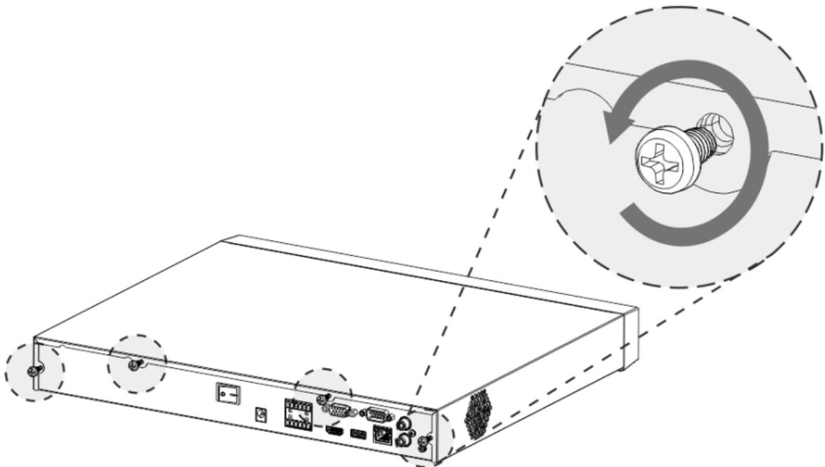
Step 2 Remove the case cover along the direction shown in the following arrow.
