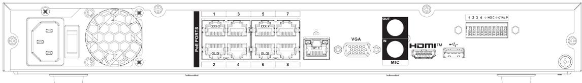
The NVR42-16P-4KS2/NVR42-16P-4KS2/L series rear panel is shown as below.
