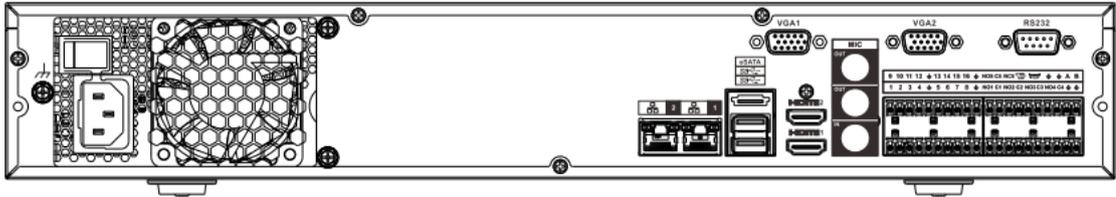
The NVR54-16P-4KS2/NVR58-16P-4KS2 series rear panel is shown as below.
