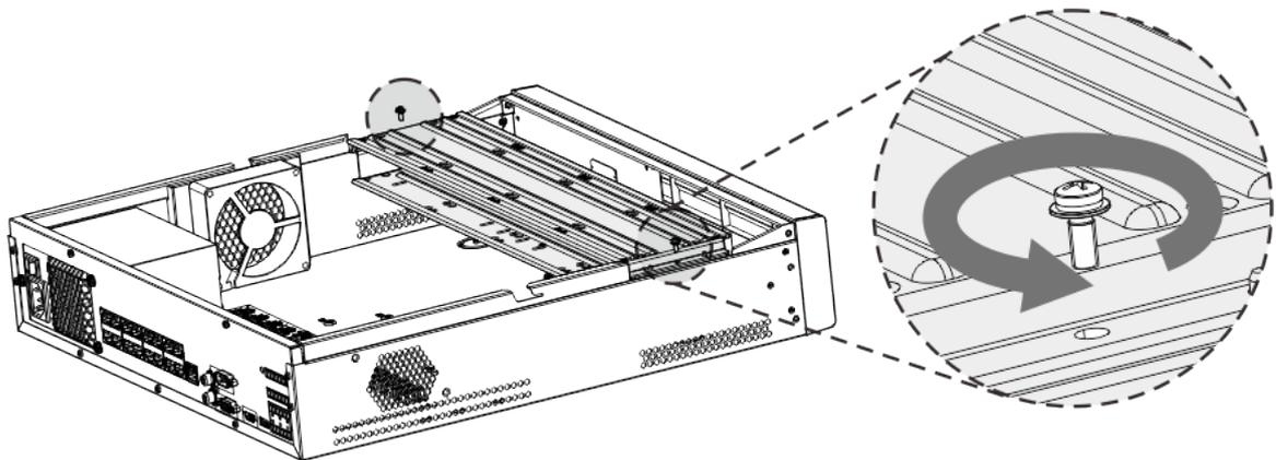
**Step 4** Match the four screw holes on the HDD with the four holes on the bracket and then fasten the screws.
