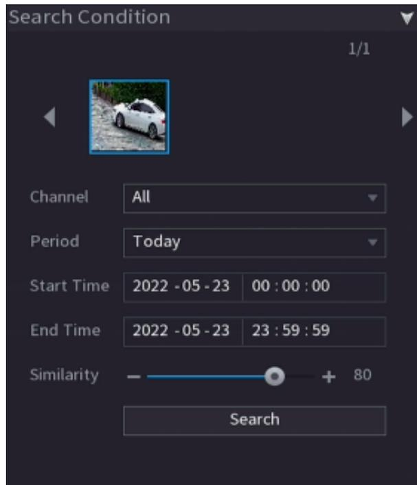
Step 5 Hover over a search result to view the basic information including channel, start time, end time and target type. Double-click a result to play the video.
