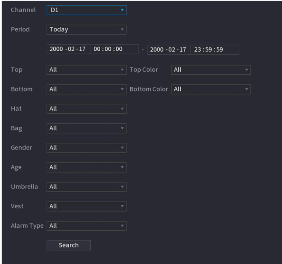
Step 2 Select a channel, start time, end time, and set corresponding parameters.
