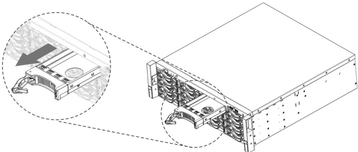
**Step 2** Put the HDD into the HDD box along the direction shown in the following arrow.
