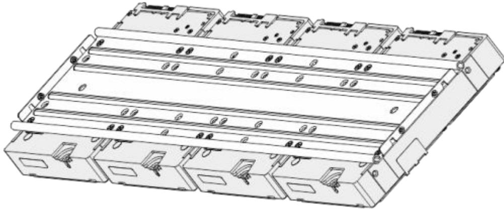
Step 6 Lock the two HDD brackets.
