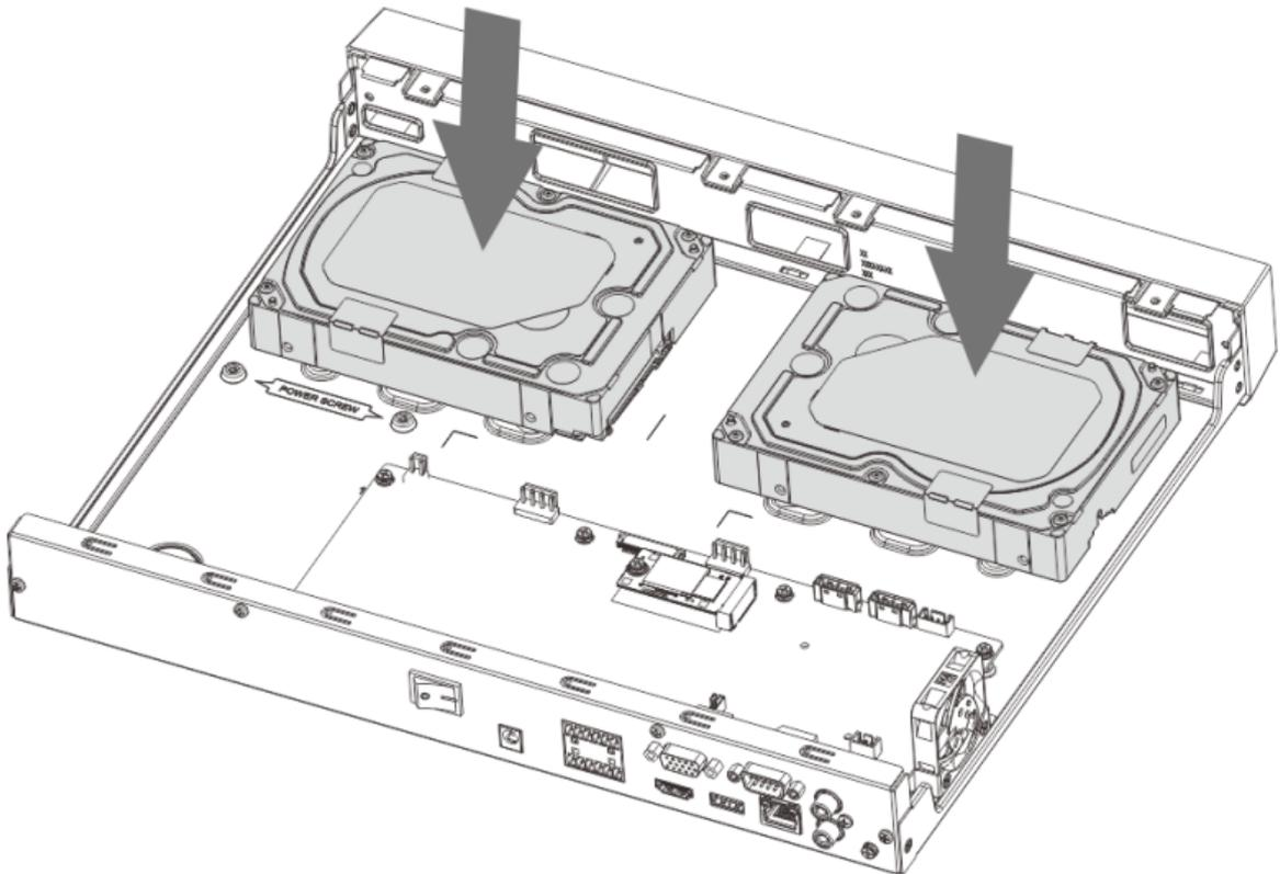
**Step 4** Turn the device upside down, match the screws with the holes on the HDD and then fasten them. The HDD is fixed to the baseboard.
