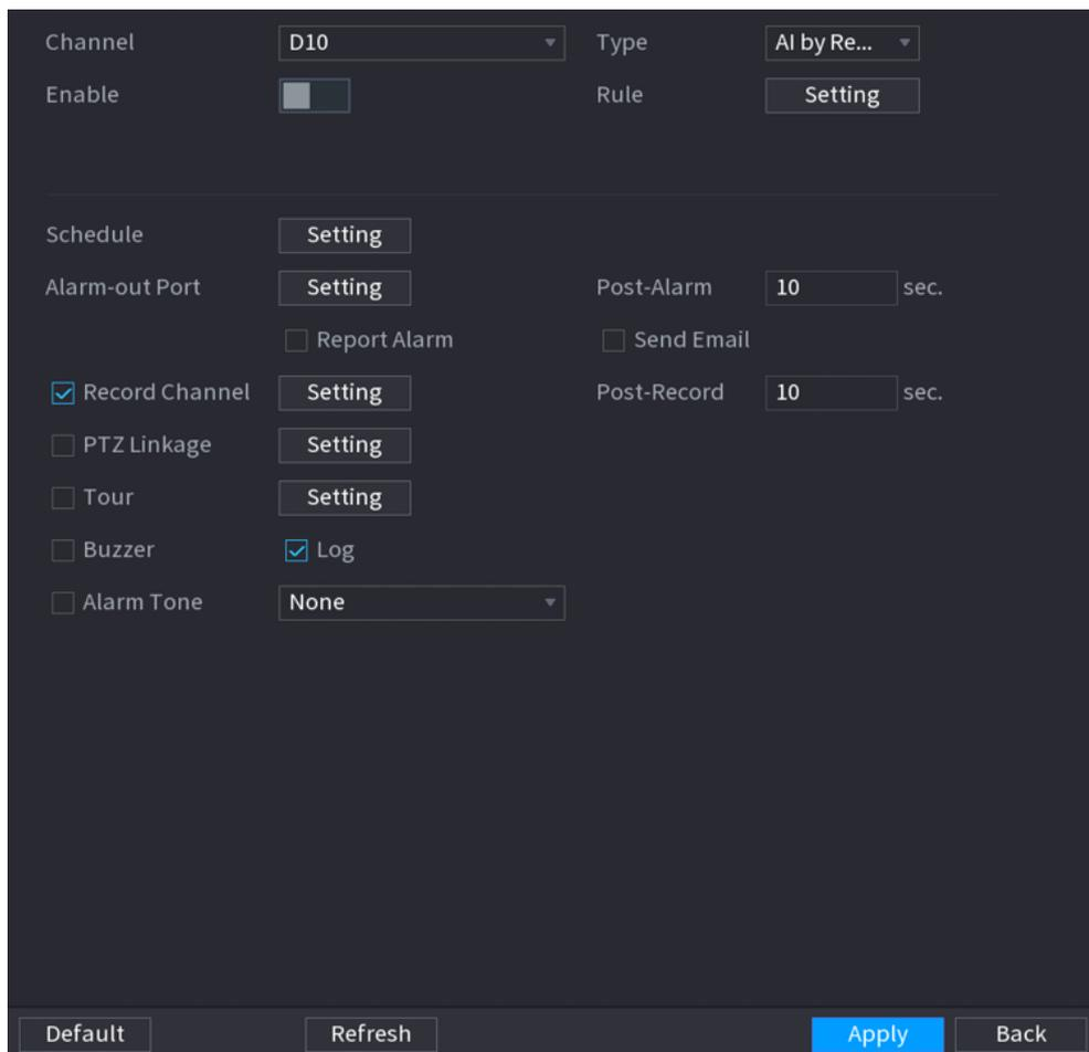
Step 2 Select a channel, and then select **AI by Reorder** or **AI by Camera** as **Type**.
