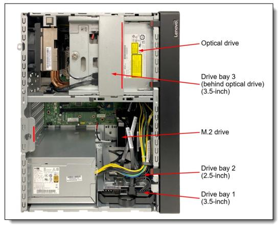
Figure 7. ST50 V2 drive bays (side view)
