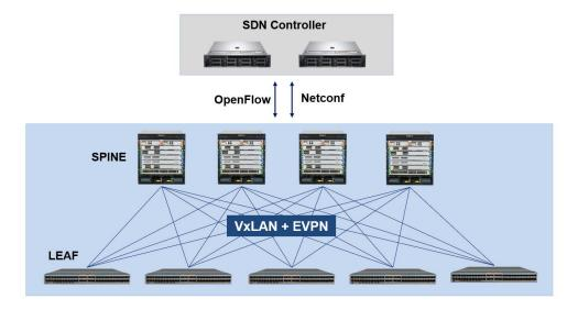
Fabric architecture has become a common and popular design option for building new-generation enterprise data center networks. Virtual Extensible LAN (VXLAN) and Ethernet VPN (EVPN) is essentially becoming the standard technology used for deploying network virtualization overlays in data center fabrics.
