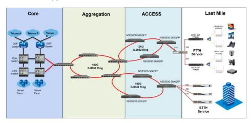
With the rapid growth of triple-play services, higher requirements are put forward for the performance, bandwidth and quality of the ISP Metro Ethernet networks. The NSS18500 series 100G core switch have been developed to meet the increasing demand of FTTx services for ISPs. The NSS18500 series provide up to 288-Port 100G interfaces for building backbone network. It will greatly increase the bandwidth and improve the internet experience of end users.
